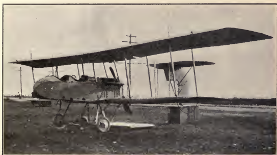
FIG. 10.—An American pusher biplane design.
