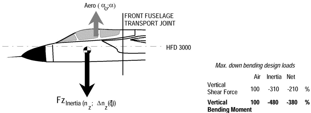
**Conclusion: An increasing Front Fuselage mass will lead to higher Front Fuselage loading.**
