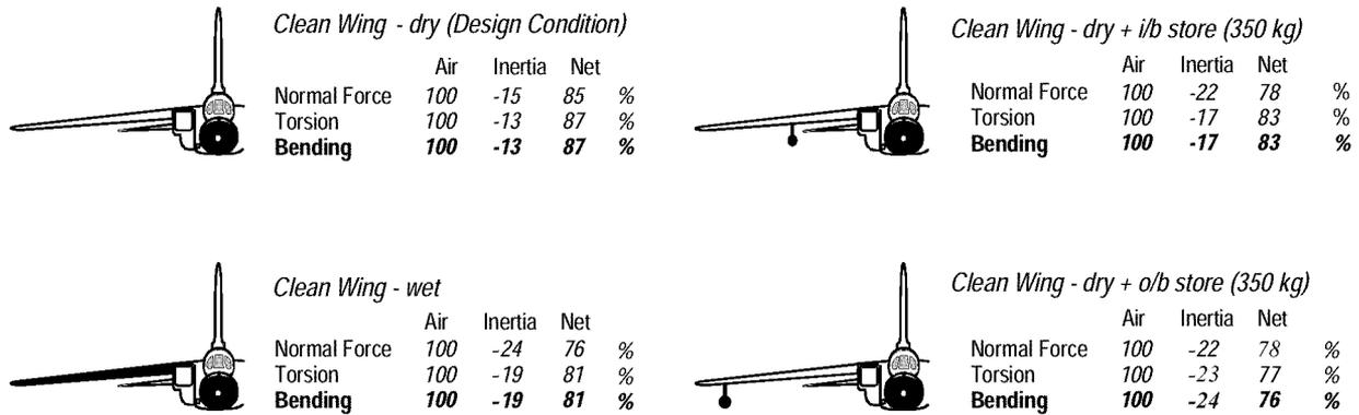
**Conclusion: Adding mass to the wing (e.g. carriage of stores) leads to reduced wing loads.**
