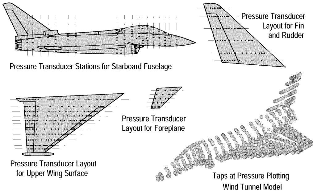
**Fig. 1.4- 1 Prototype Pressure Plotting for Flight Load Survey**
