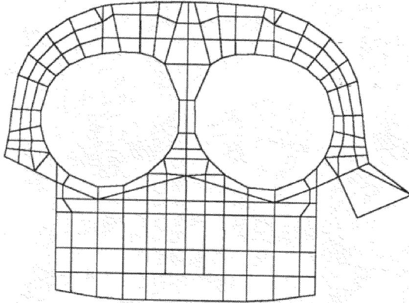
**Fig. 2.2-4A Coarse Mesh FE-Model of Center Fuselage Frame**
