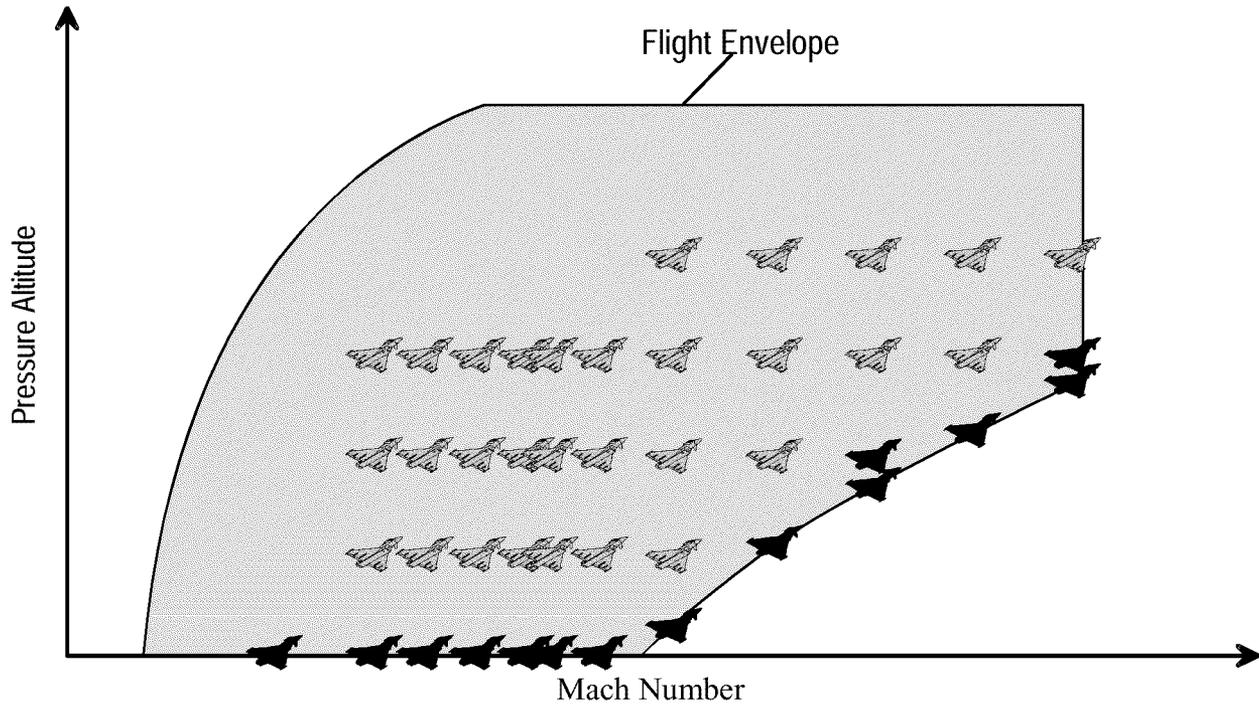
**Fig. 1.2.1-3 Mach - Altitude Points of Loads Model (flex. Aerodynamics)**
