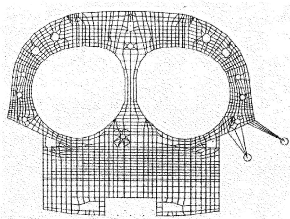
**Fig. 2.2-4B Fine Mesh FE-Model for Detail Analysis**
