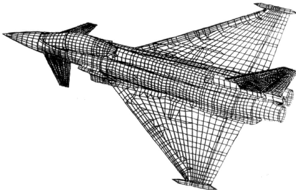
**Fig. 2.2-3 EF2000 Global Model for Unified Analysis**
