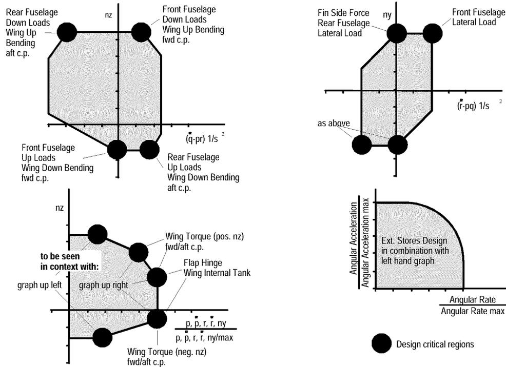
**Fig. 1.2.3-2 Flight Parameter Envelopes for Structural Design**
