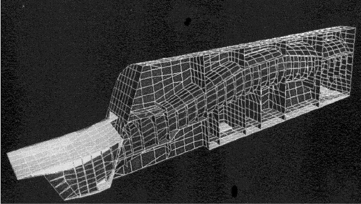
**Fig. 2.2-2 FE-Half-Model of Center Fuselage Structure**
