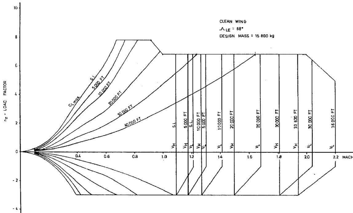
**Fig. 1.2.1-1 Ma-n Diagram in Altitude**
