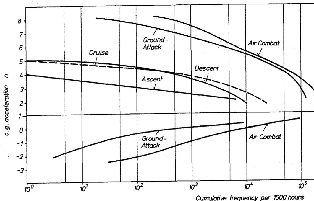
**Fig. 2.1- 2 Typical Excedance Curves for Combat Aircraft**
