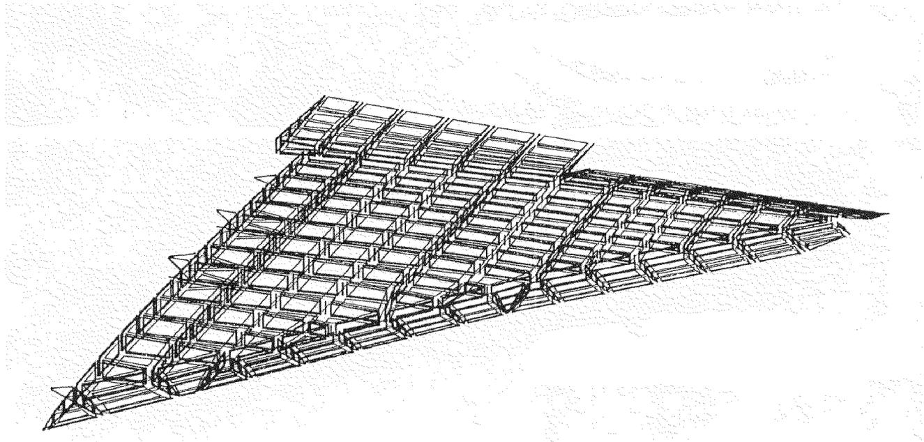
**Fig. 2.2-1 Coarse Mesh FE-Model of Wing Structure**
