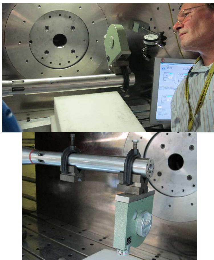
Figure 10: 120 mm clinometer measuring the arbor roll angle
