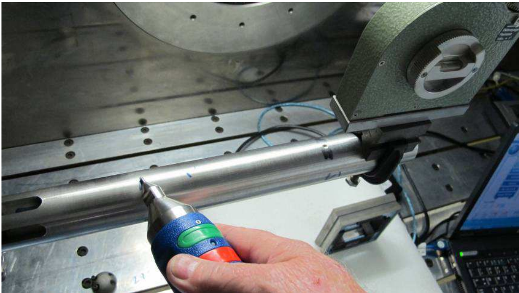
Figure 6: CMM measuring the arbor vertical position in the test section
