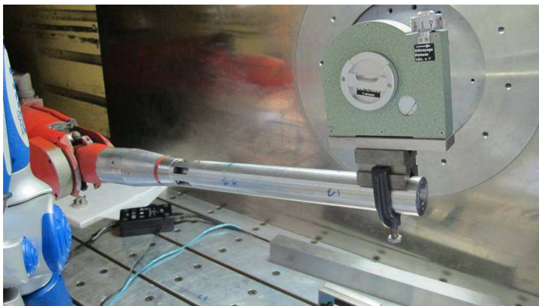
Figure 9: 120 mm clinometer measuring the arbor pitch angle
