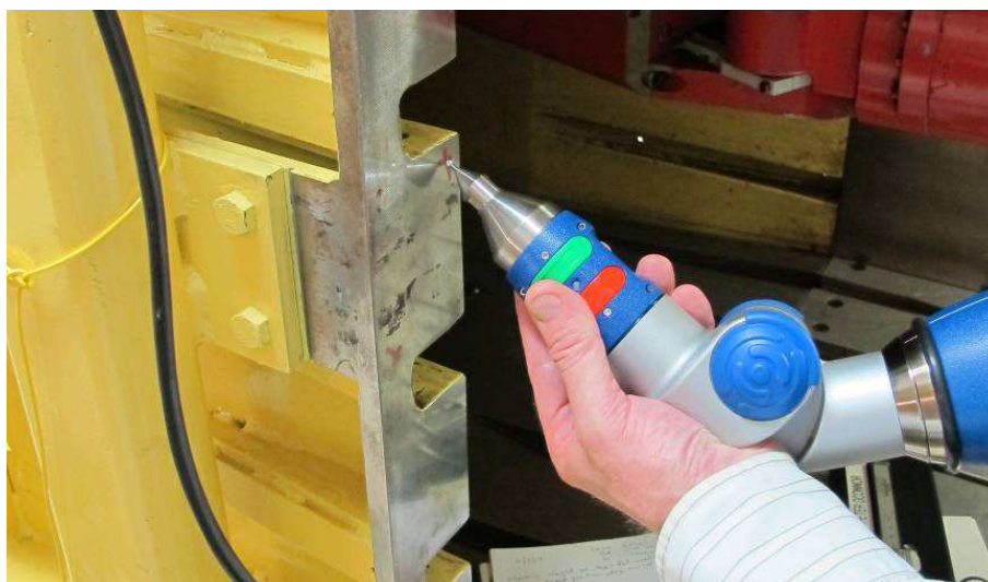
Figure 4: CMM measuring the STA 6205 reference face
