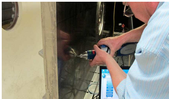
Figure 14: CMM measuring the width of the test section
