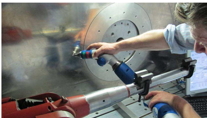
Figure 13: CMM measuring the inner sidewall reference plane
