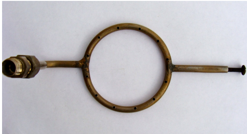
Figure 1. Exhaust gas sampling ring
