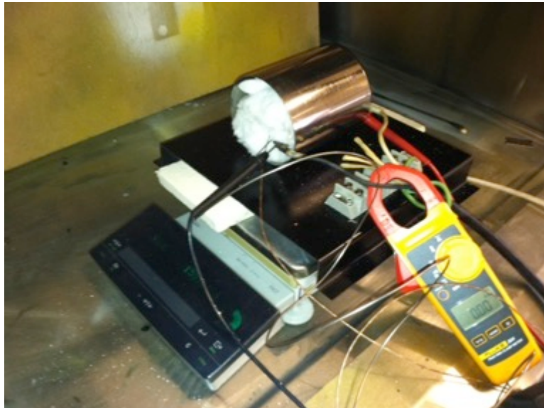
Figure 3. Experiment in thermal capacitance calorimeter
