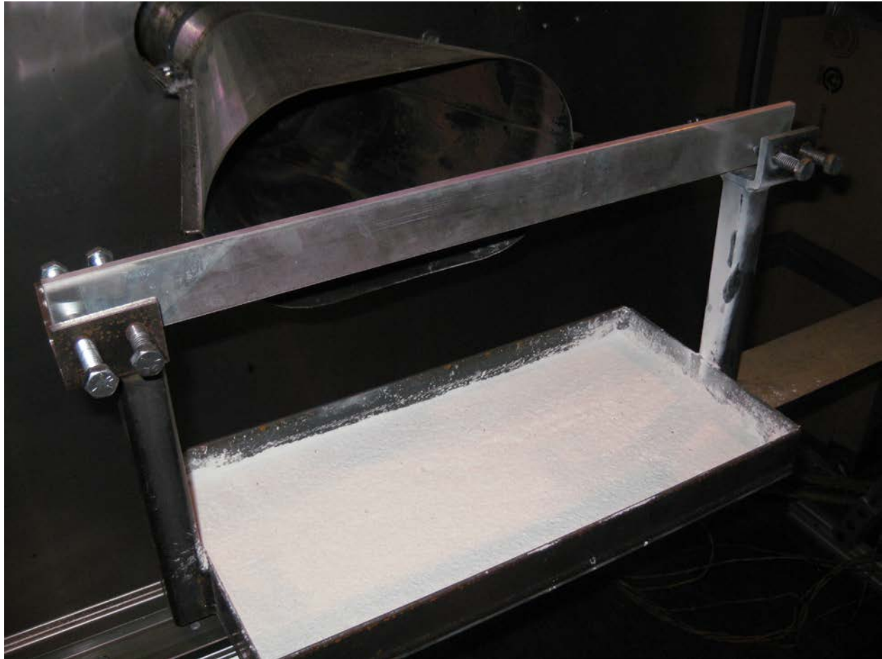
Figure 119. Updated Horizontal Bar Sample Holder
