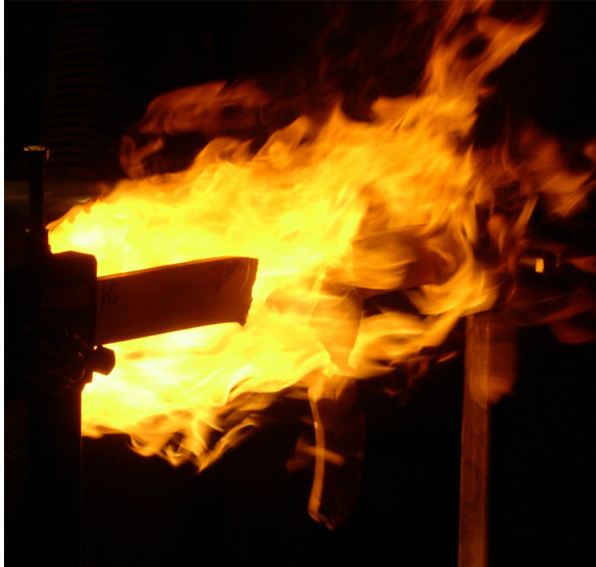
Figure 5. Center Section of WE43 Bar Sample Falling Into Catch Pan After Melting
