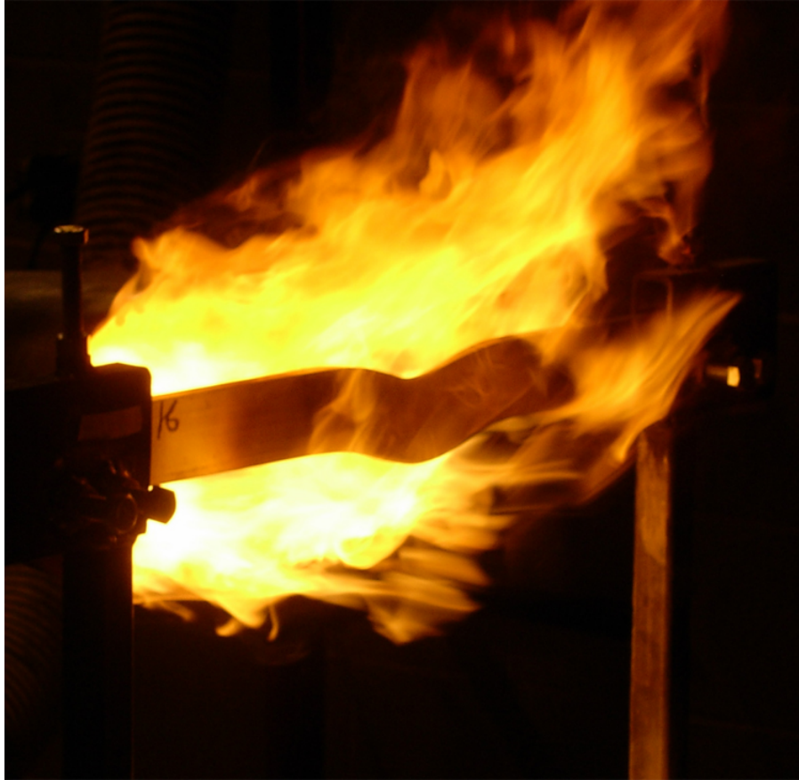
Figure 4. Magnesium Alloy Bar Sample Immersed in Flames, Just Prior to Melting
