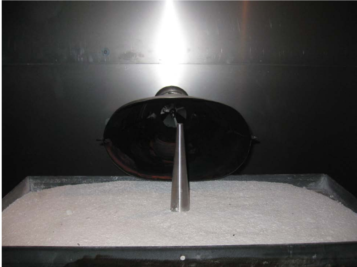
Figure 45. Shortened Truncated Cone Sample With Burner Shown in Background (3/28/2011)
