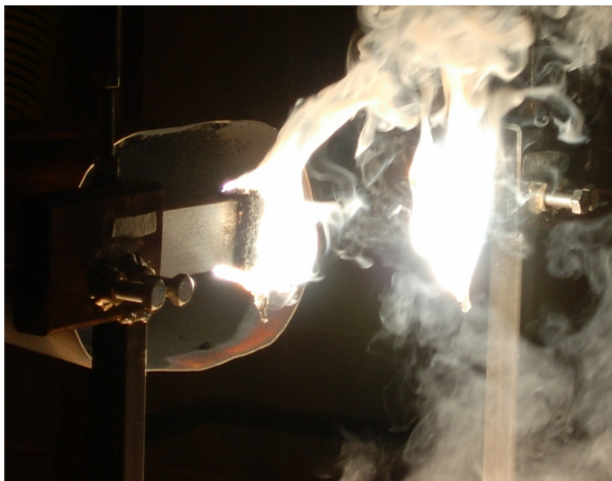
Figure 6. Ignition of Magnesium Alloy AZ31 Following Burner Flame Exposure
