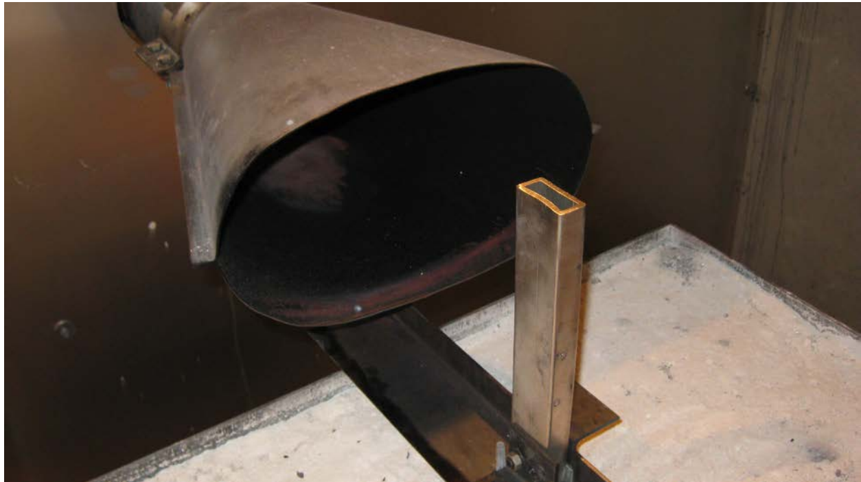
Figure 95. Vertically Oriented Rectangular Cross-Section Sample (10/6/2011)
