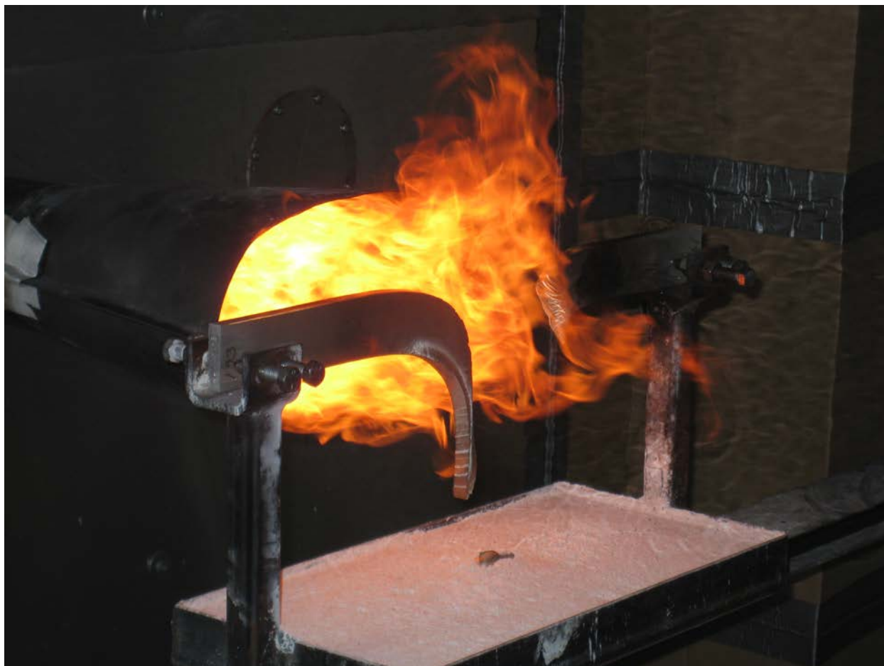
Figure 128. Sample Material Melting and Rotating Into Catch Pan Below
