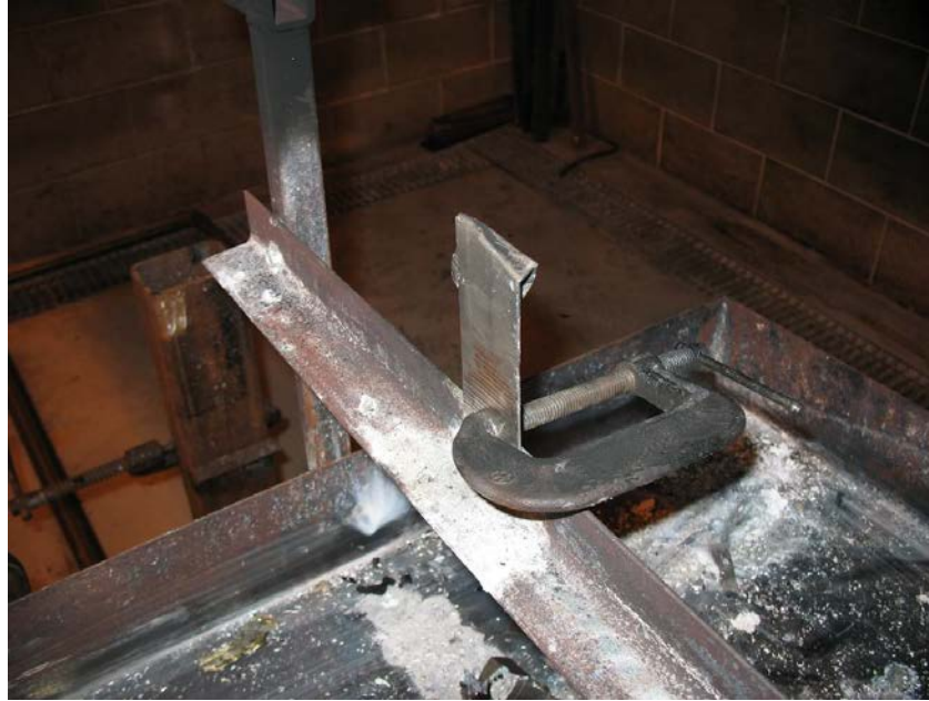
Figure 19. Vertically Mounted Slice After Self-Extinguishment
