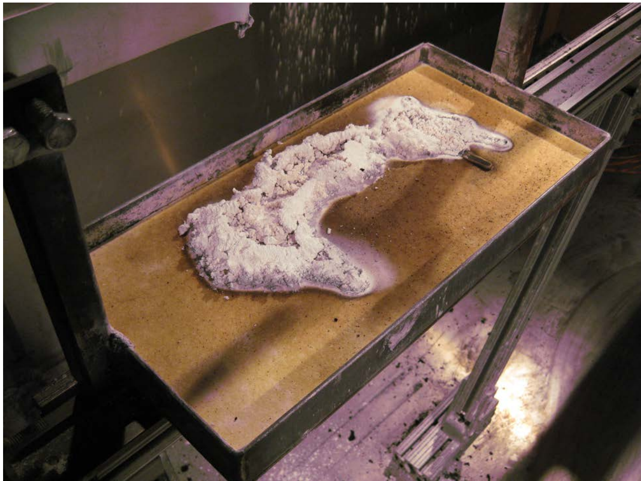
Figure 137. The ZE41 Test Result Using Kaowool™ Board in Catch Pan (2/20/2013)
