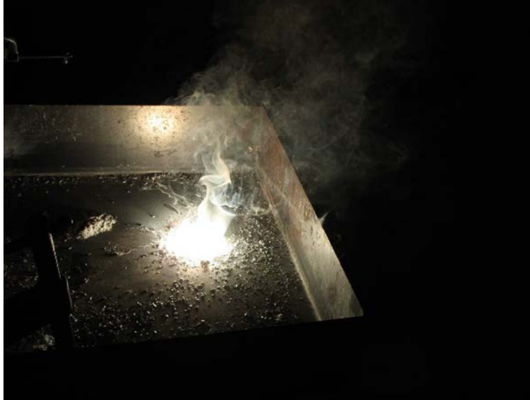
Figure 15. Small Pile of Magnesium Alloy Millings on Fire
