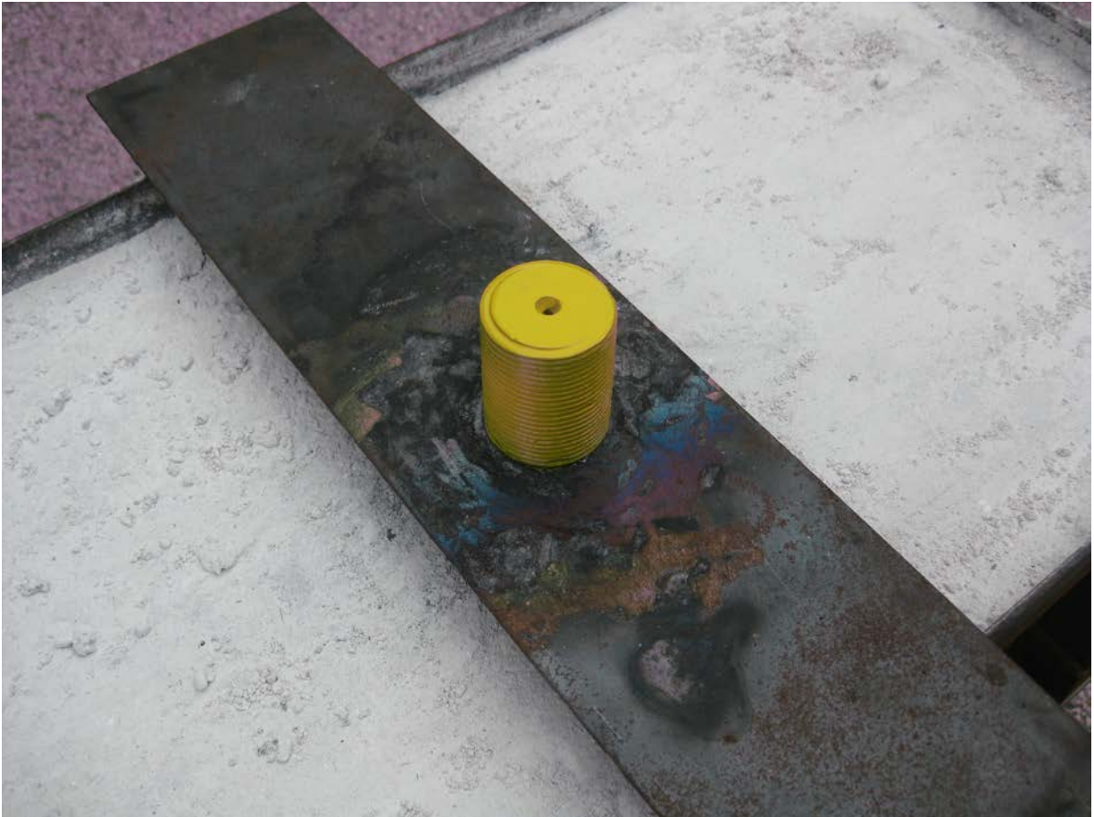
Figure 110. Sample Holder Used for 1.75-Inch OD Samples With 0.125-Inch Wall Thickness
