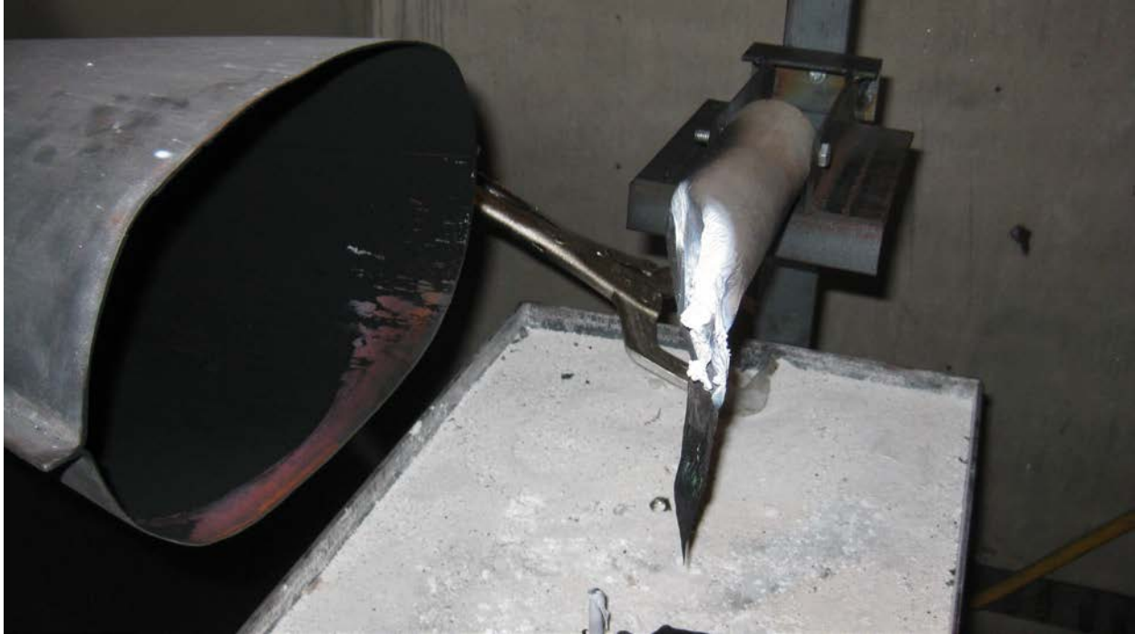
Figure 81. Side View of Horizontally Mounted Cylindrical Tubing Sample, Post-Test (9/30/2011)
