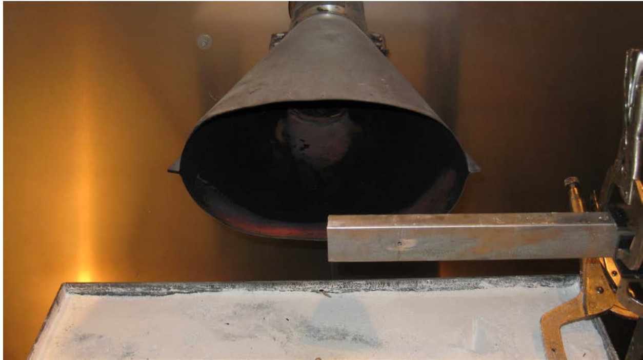
Figure 60. Rectangular WE43 Box Section Component Mounted Horizontally, Front View (9/22/2011)
