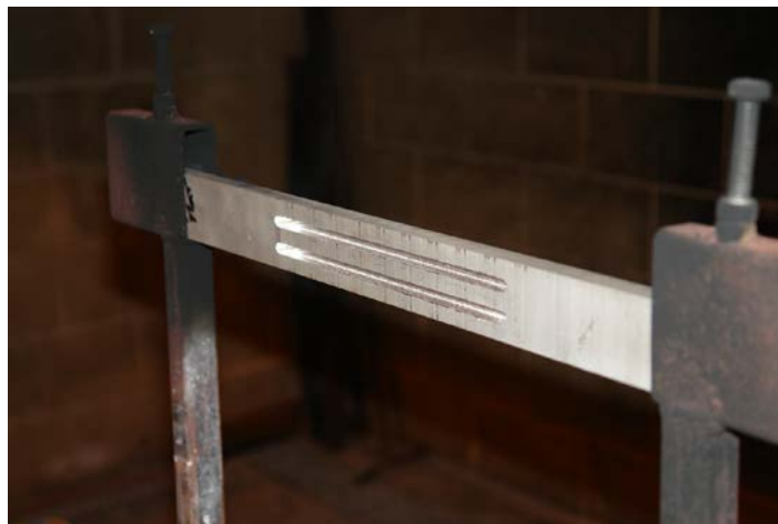
Figure 10. Magnesium Alloy Test Sample Bar With a Milled Cross Section
