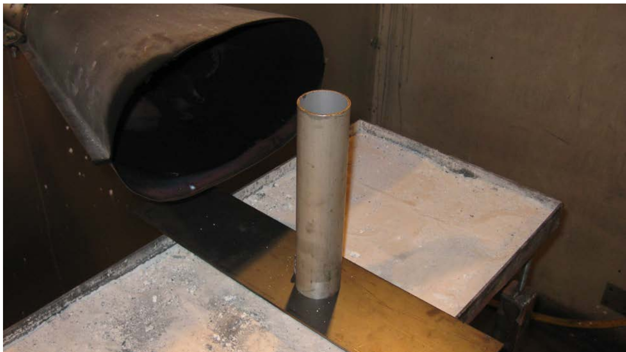
Figure 88. Vertically Mounted OEM Aluminum Cylindrical Tubing Sample (10/03/2011)
