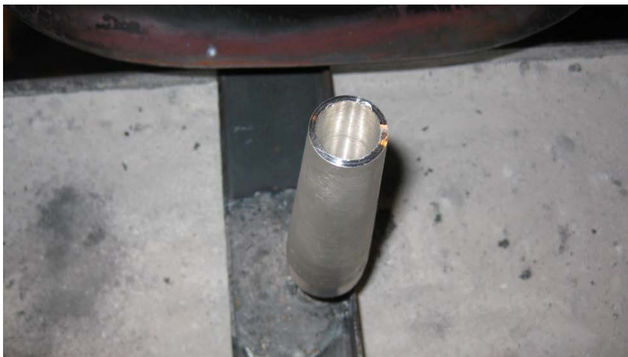
Figure 98. Closeup of Specially Prepared Truncated WE43 Cone Sample With Center Bore (10/11/2011)
