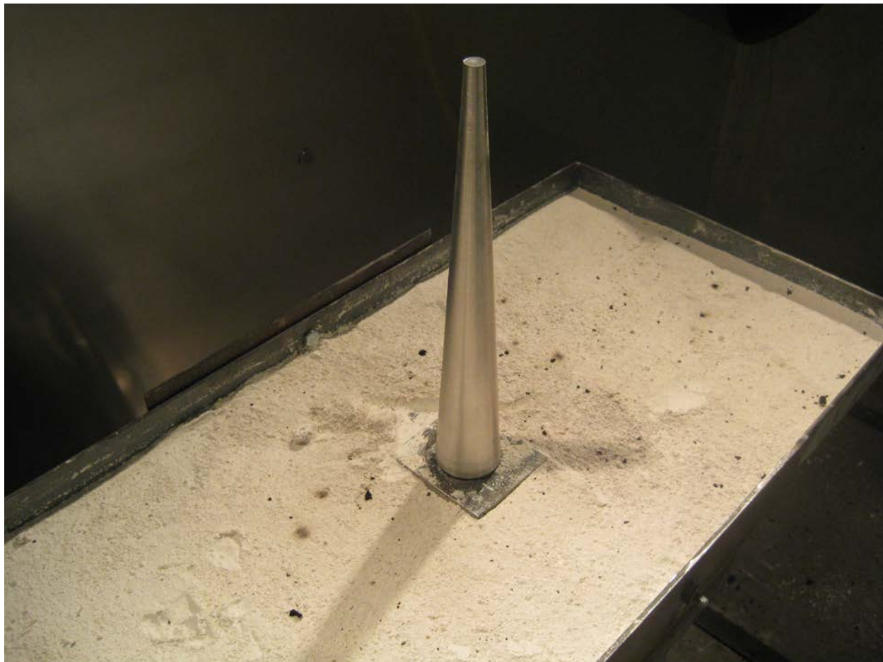
Figure 36. Truncated Cone-Shaped Test Sample Affixed in Talc-Filled Catch Pan (2/8/2011)
