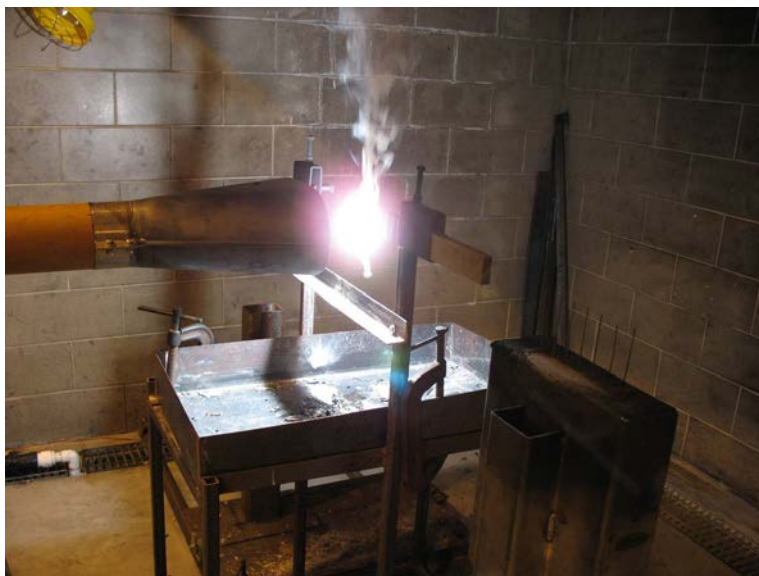
Figure 21. Sectioned Magnesium Alloy Bar Sample Ignited Using Oil Burner
