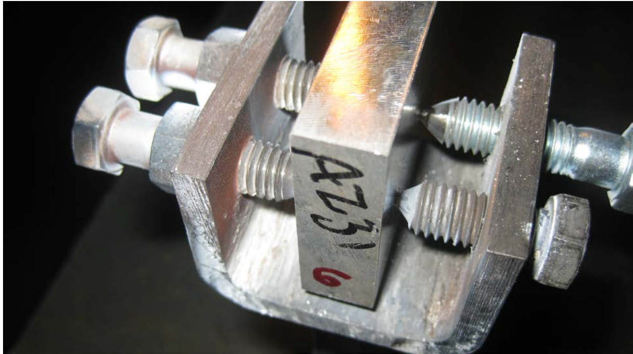
Figure 120. Updated Sample Securing Mechanism
