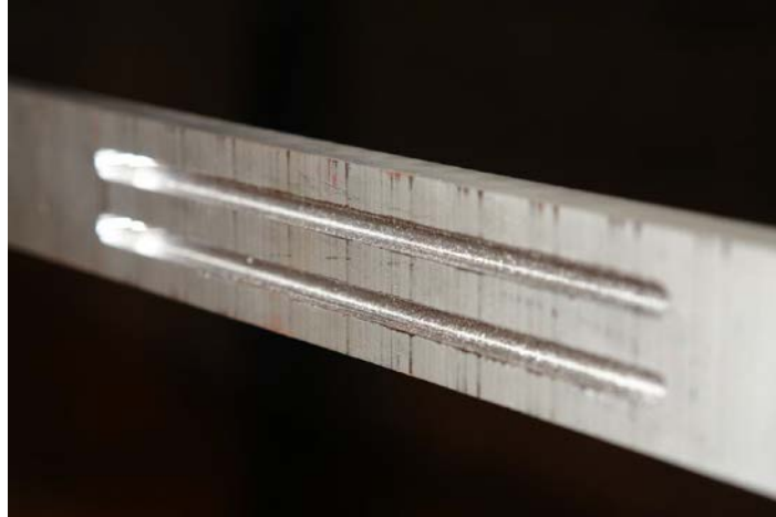
Figure 11. Close-up of Test Sample Bar With a Milled Cross Section
