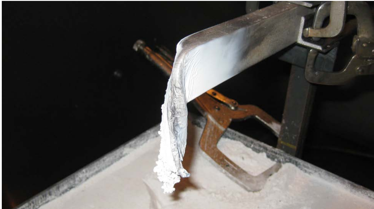
Figure 62. Rectangular WE43 Box Section Component, Post-Test (9/22/2011)
