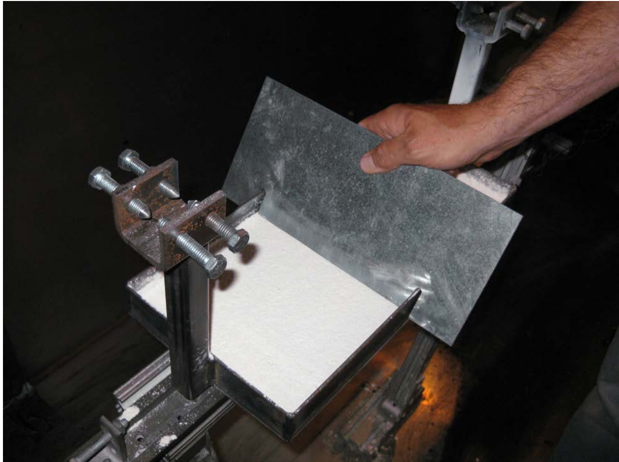
Figure 121. Screeding Device Used to Level off Layer of Talc in Catch Pan
