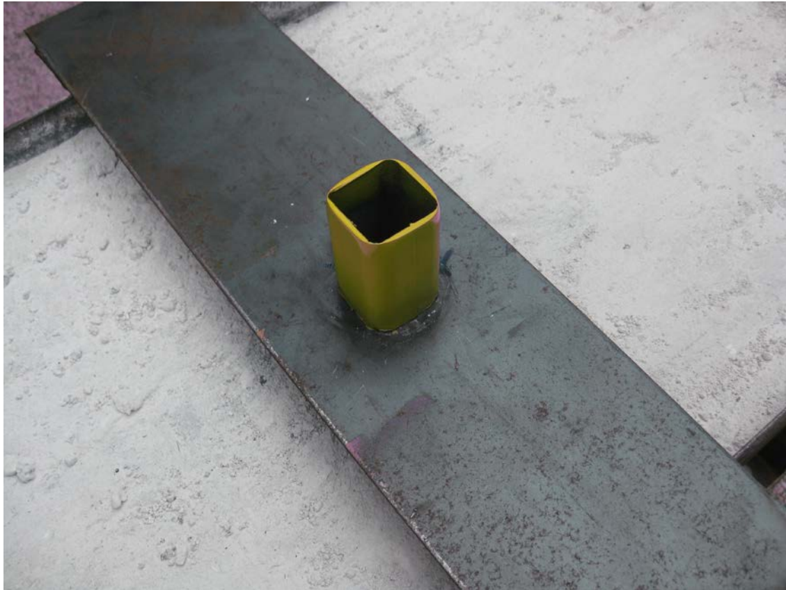
Figure 84. Box Tubing Stub Holder for Cylindrical Sample
