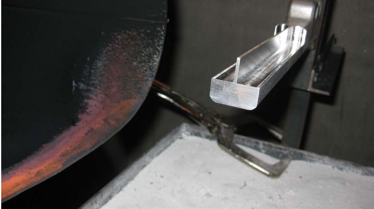
Figure 71. Thin T-Beam Cross-Section Sample Machined From Seat-Leg Component (9/28/2011)
