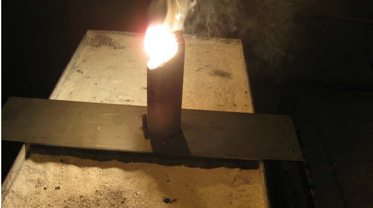
Figure 102. Flaming of Vertically Mounted Cylindrical Tubing Sample After Burner Removal (10/12/2011)
