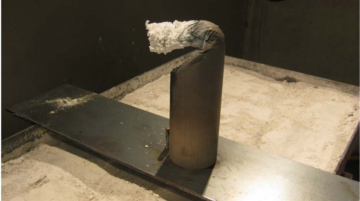
Figure 86. Side View of Vertically Mounted Cylindrical Tubing Sample, Post-Test (9/30/2011)
