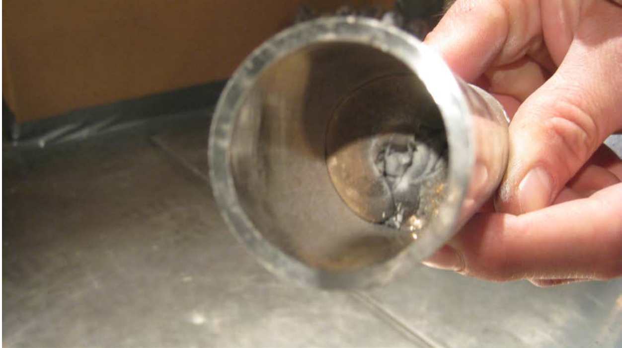
Figure 116. Post-Test Inspection of Sample Bottom Showing Collection of Molten Material
