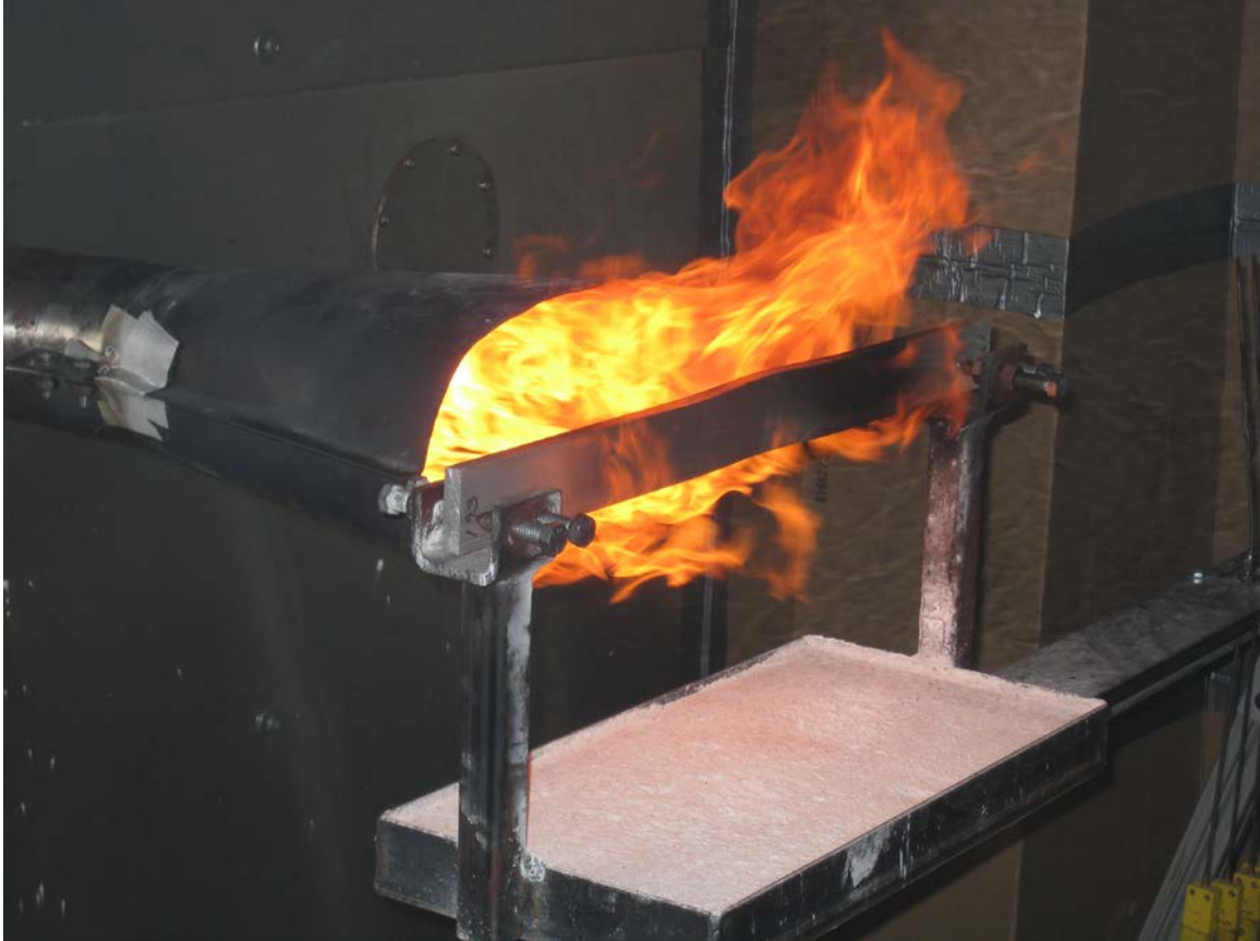
Figure 131. Test Showing a Talc Depth of Approximately 1 Inch
