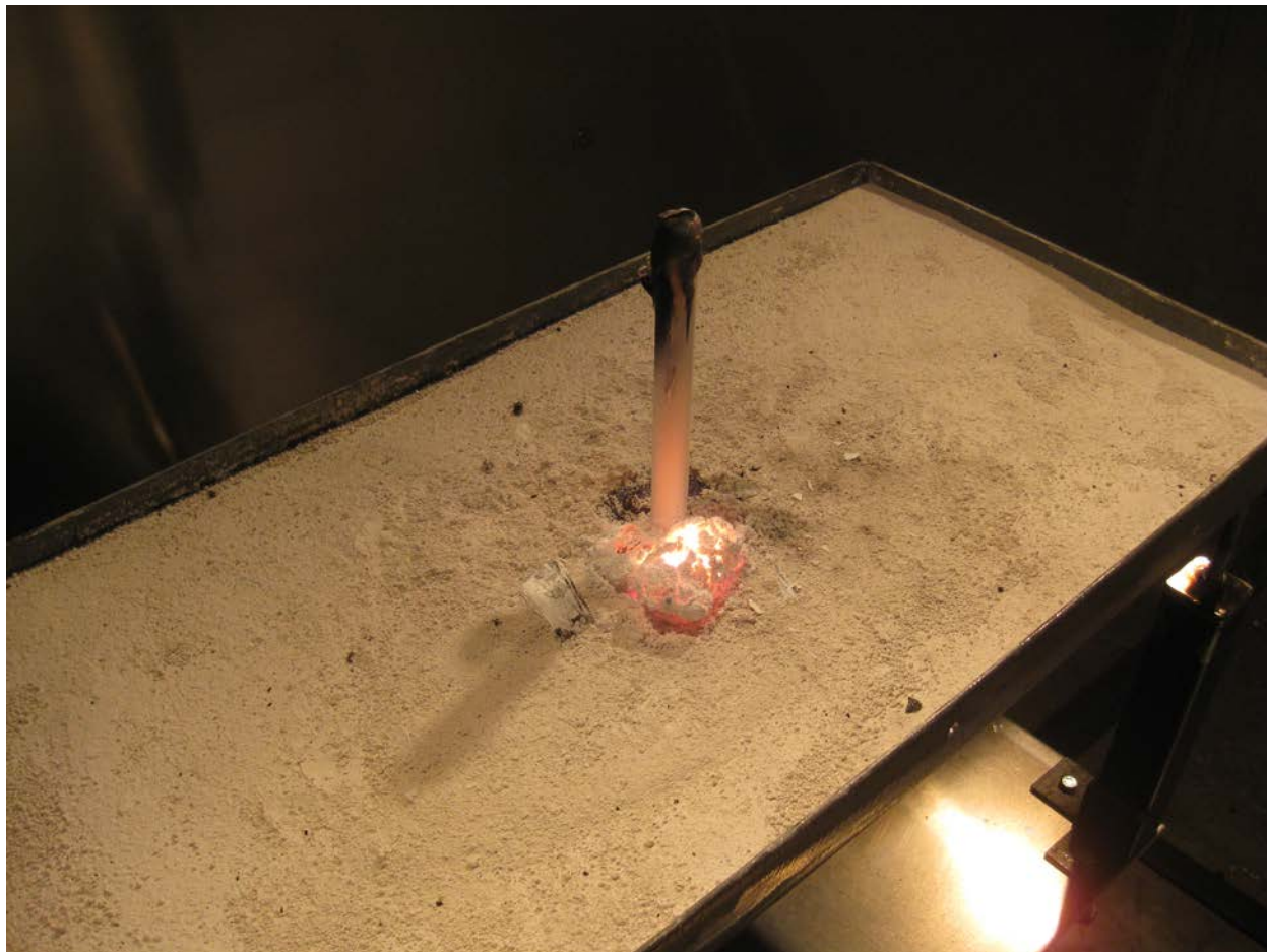
Figure 41. Cylinder-Shaped Test Sample Showing Large Segment Separating and Falling Into Talc-Filled Catch Pan (2/24/2011)
