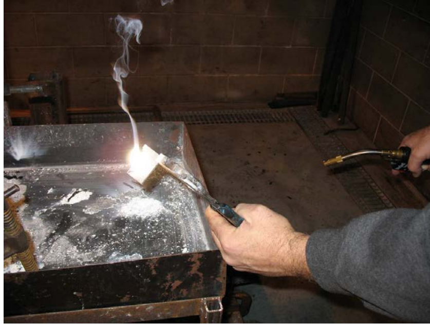
Figure 17. Thin Sliver of Magnesium Alloy on Fire After Being Heated With Torch
