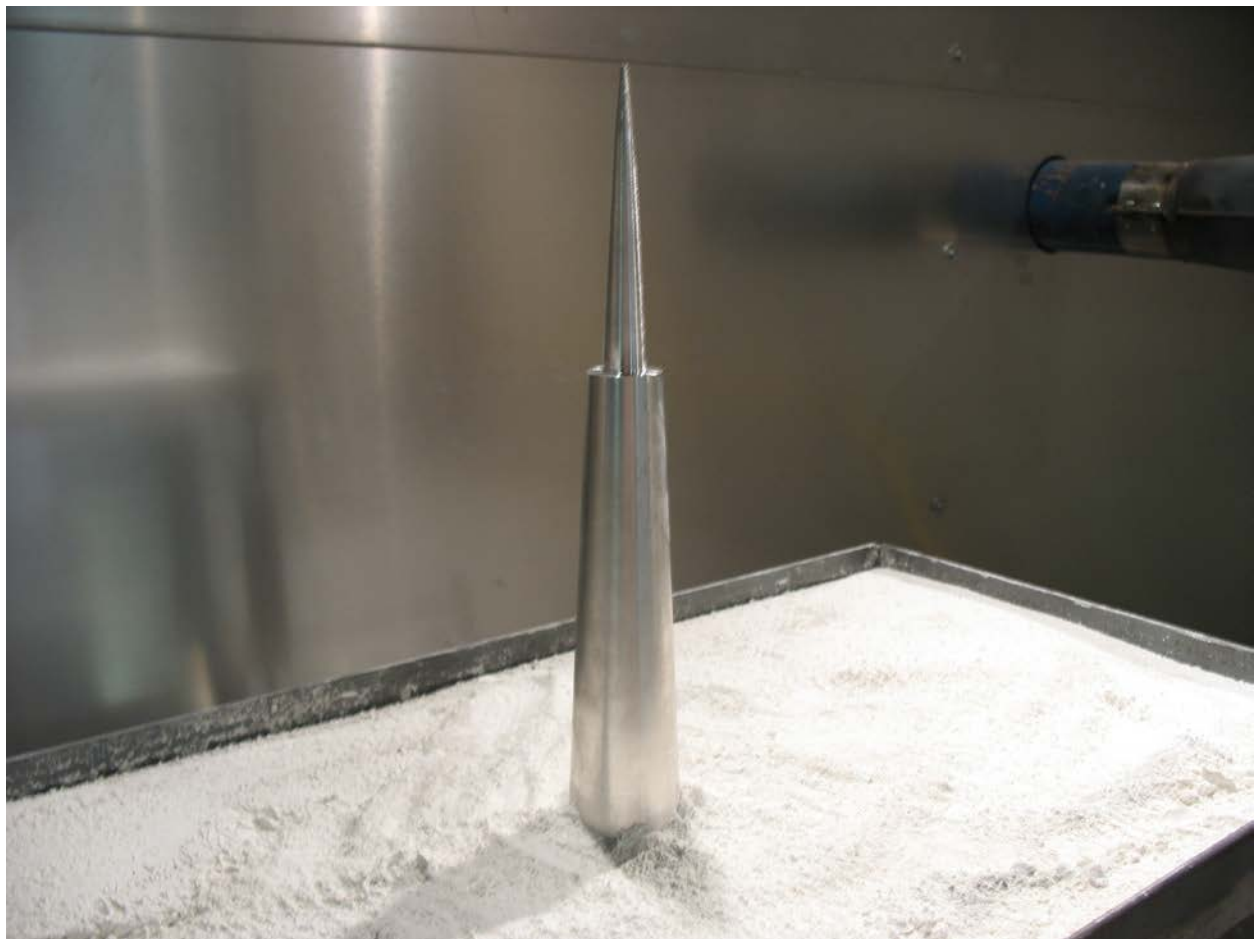
Figure 42. Conical Step-Shaped Test Sample Affixed in Talc-Filled Catch Pan (3/22/2011)
