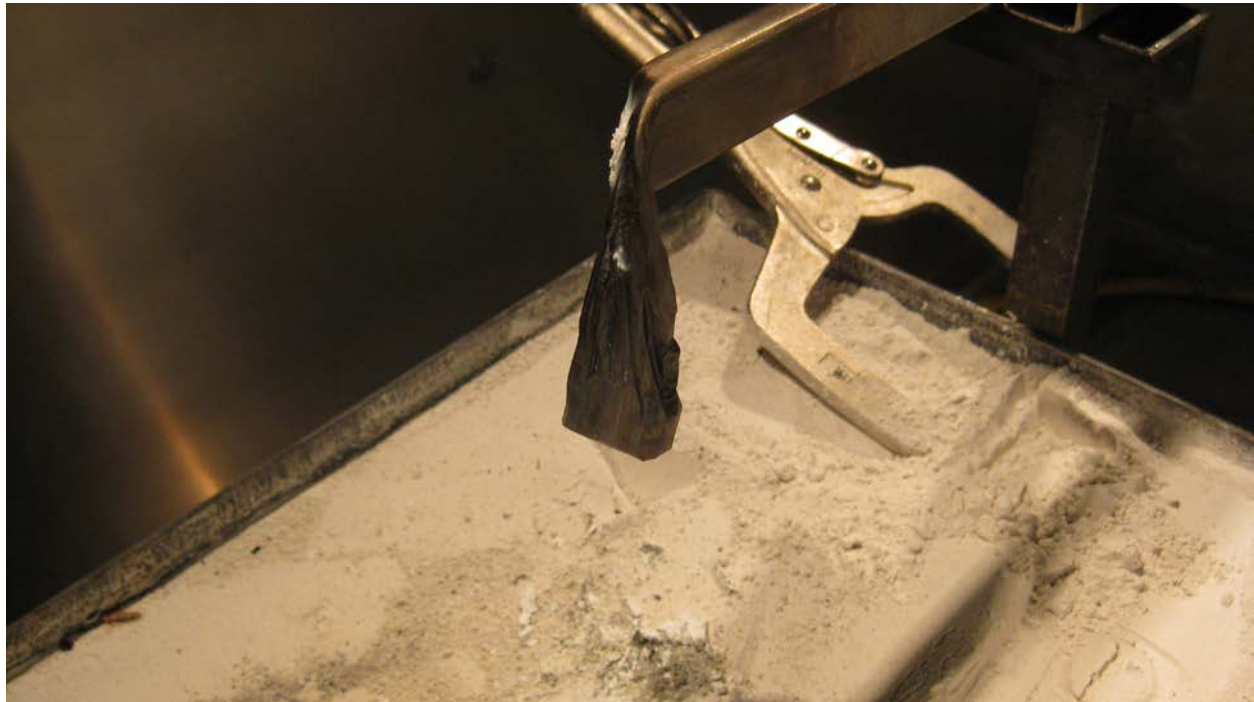
Figure 65. Smaller Rectangular WE43 Box Section Component, Post-Test (9/22/2011)
