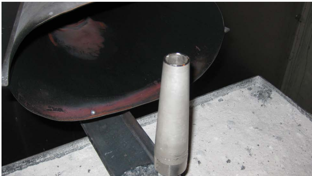
Figure 97. Specially Prepared Truncated WE43 Cone Sample With Center Bore (10/11/2011)
