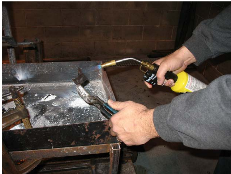
Figure 16. Thin Sliver of Magnesium Alloy Being Heated With Torch
