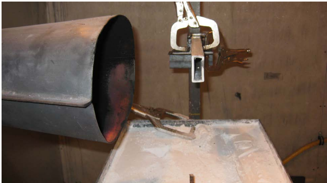
Figure 61. Rectangular WE43 Box Section Component Mounted Horizontally, Side View (9/22/2011)
