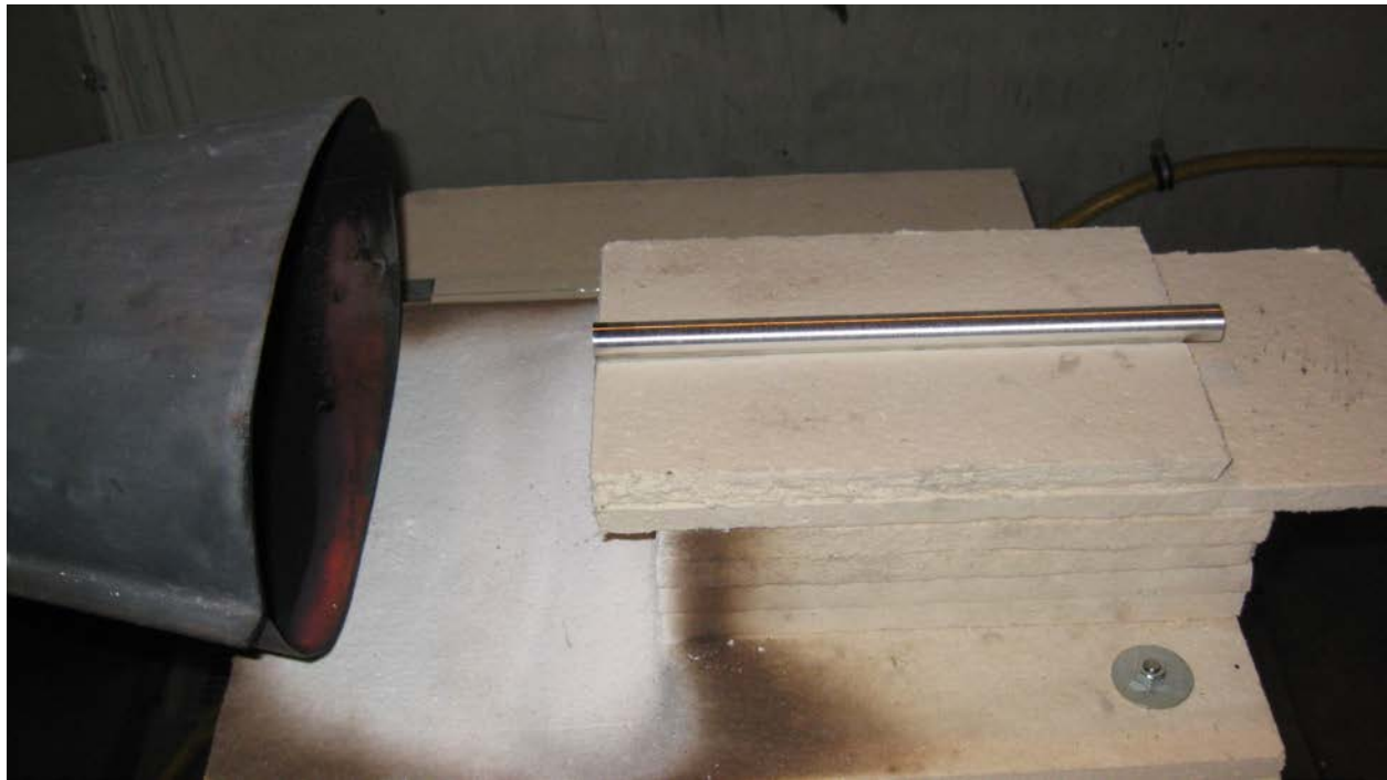
Figure 58. Thin Horizontal AZ31 Cylinder Sample on Grooved Ceramic Boards (9/21/2011)
