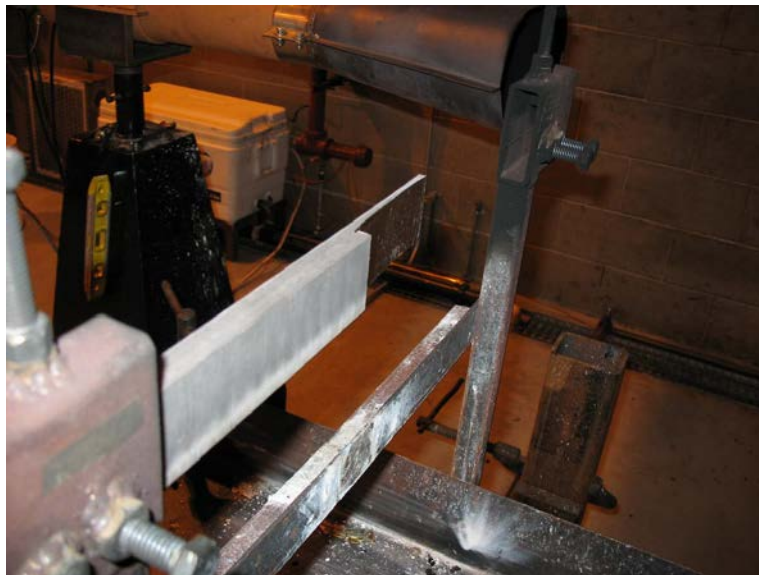
Figure 20. Sectioned Bar Sample Positioned Horizontally in Front of the Burner
