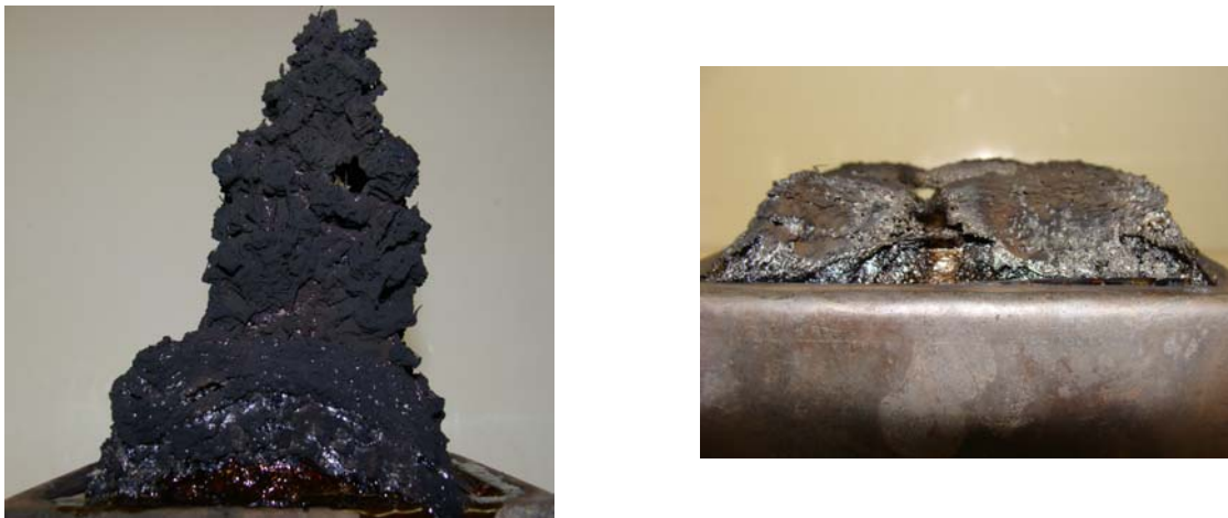
Figure 3. Photographs of 6-mm-Thick Samples of PC (left) and PVC (right) Burnt in the Cone Calorimeter at EHF_0 = 75 \text{ kW m}^{-2} (Both tests were stopped at about 200 s; the samples were removed from under the cone heater and photographed.)
