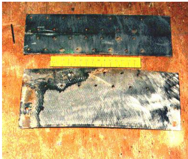
Figure 14. Photograph of Patch That Suffered Adhesion Failure in Service
