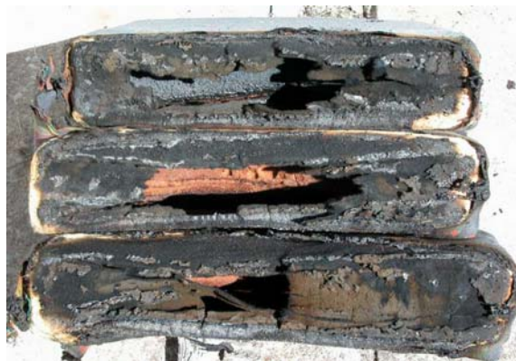
Figure 5. Fire-Blocking Layer; Horizontal Cushions
