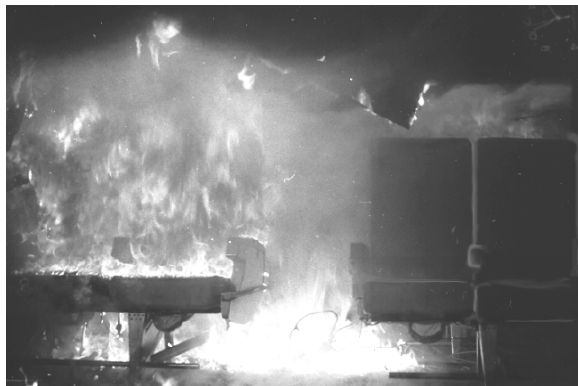
FIGURE 1. FULL-SCALE FIRE TEST SHOWING SEAT CUSHION INVOLVEMENT
