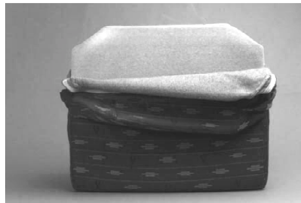
FIGURE 2. AIRCRAFT SEAT CUSHION INCLUDING COVER FABRIC, FIRE- BLOCKING LAYER, AND POLYURETHANE FOAM CUSHION
