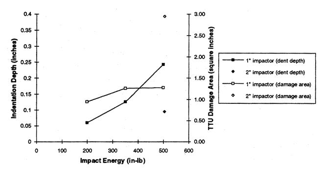
FIGURE 14. IMPACT DAMAGE RESISTANCE OF BASELINE AFT KEEP SANDWICH STRUCTURE
