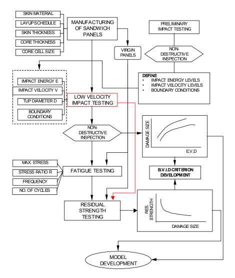
FIGURE 28. SUMMARY OF THE DAMAGE RESISTANCE AND TOLERANCE INVESTIGATION OF SANDWICH PANELS
