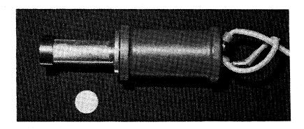
FIGURE 11. A TYPICAL LOW-MASS IMPACTOR
