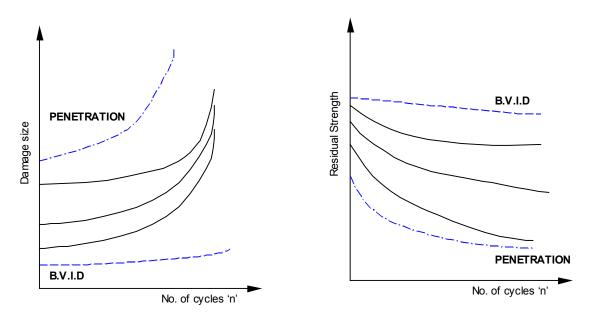
FIGURE 27. TYPICAL DAMAGE GROWTH AND RESIDUAL STRENGTH CHARACTERISTICS FOR SANDWICH PANELS WITH VARIOUS INITIAL FLAW SIZES/TYPES
