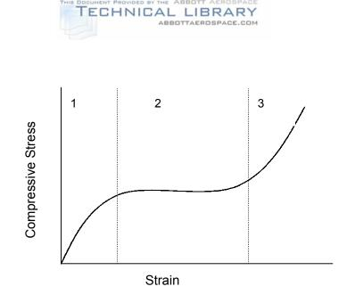
FIGURE 5. IDEALIZED COMPRESSIVE STRESS-STRAIN CURVE FOR FOAM CORE
