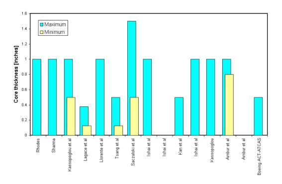
FIGURE 18. RANGES OF CORE THICKNESS USED IN PREVIOUS INVESTIGATIONS
