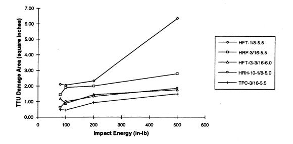
FIGURE 15. PLANAR DAMAGE AREA FOLLOWING IMPACT OF SANDWICH STRUCTURE WITH HONEYCOMB CORE MATERIALS
