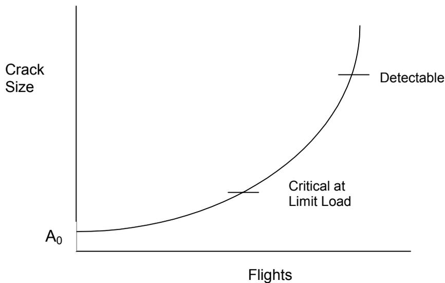
FIGURE 1. SINGLE LOAD PATH - SAFE LIFE
