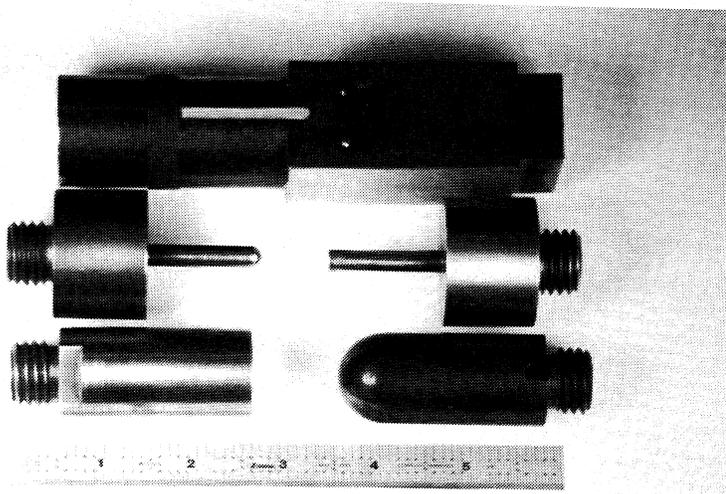
FIGURE 12. HIGH-MASS IMPACTORS USED IN THE INVESTIGATION
