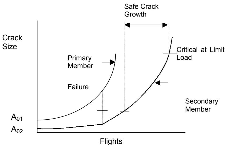
FIGURE 3. MULTIPLE LOAD PATH - EXTERNALLY INSPECTABLE
