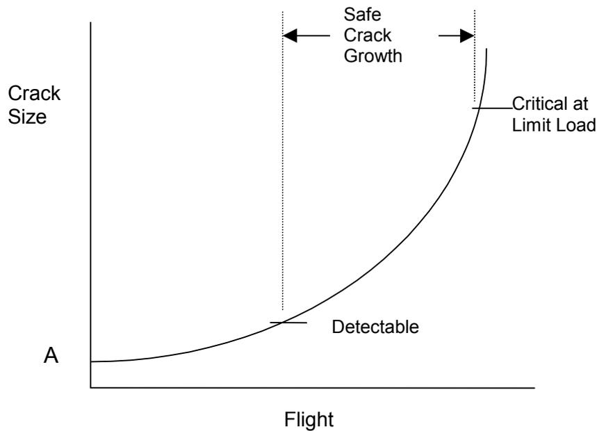
FIGURE 2. SINGLE LOAD PATH - DAMAGE TOLERANT
