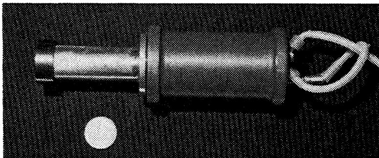
FIGURE 11. A TYPICAL LOW-MASS IMPACTOR
