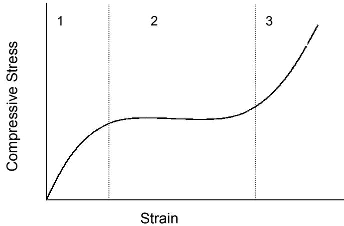
FIGURE 5. IDEALIZED COMPRESSIVE STRESS-STRAIN CURVE FOR FOAM CORE
