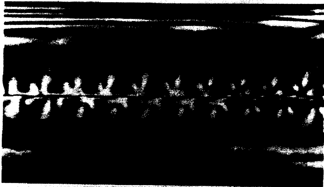
FIGURE 3.30. PHOTOELASTIC STRESS PATTERN FOR AN INDIVIDUAL E-GLASS FIBER EMBEDDED IN AN EPOXY MATERIAL
