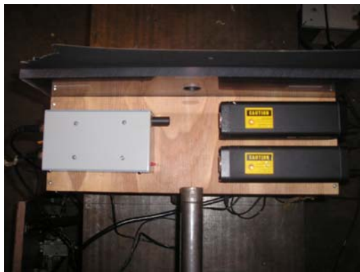
FIGURE 5. INITIAL VELOCITY MEASUREMENT SYSTEM (The photodiodes and their accompanying circuit are within the gray box.)
