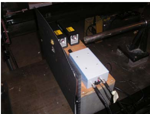
FIGURE 5. INITIAL VELOCITY MEASUREMENT SYSTEM (The photodiodes and their accompanying circuit are within the gray box.)
