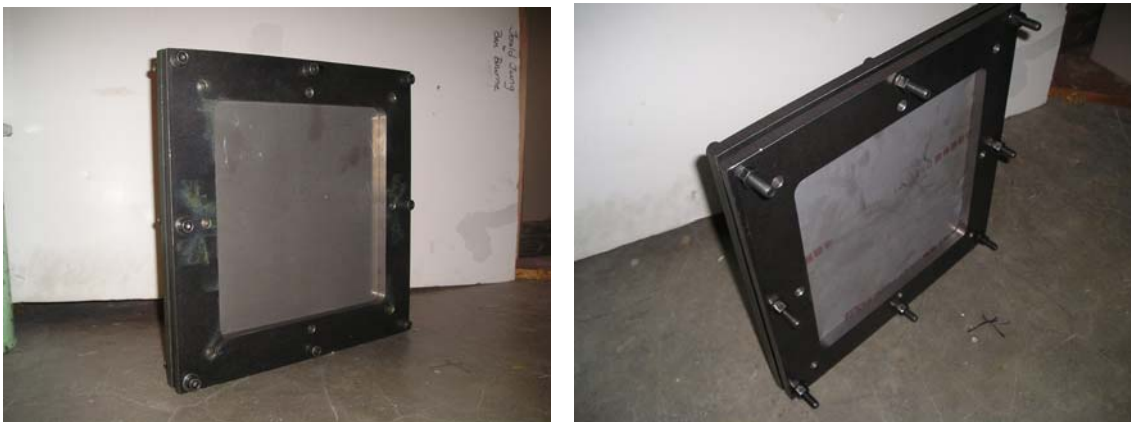
FIGURE 6. A 0.25-INCH ALUMINUM PLATE WITHIN THE TARGET HOLDER
