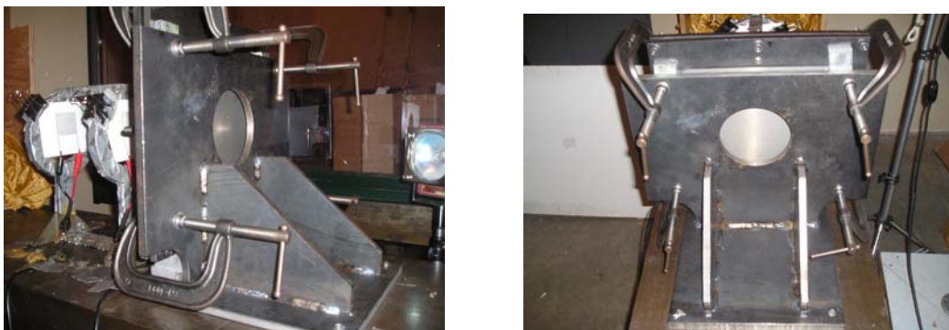
FIGURE 7. TARGET HOLDER WITH THE TARGET MOUNT ATTACHED
