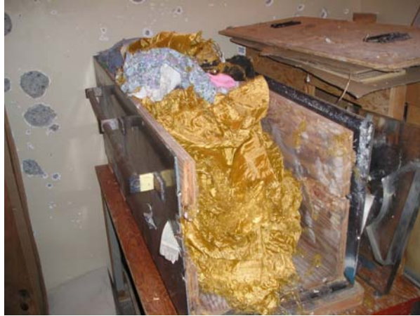
FIGURE 16. CATCHER BOX AT THE END OF THE POWDER GUN
