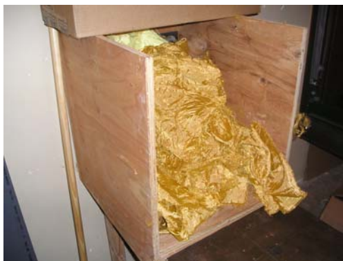
FIGURE 10. CATCHER BOX AT THE END OF THE GAS GUN
