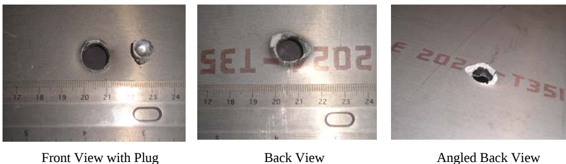
FIGURE 40. PLATE WITH AN INITIAL PROJECTILE VELOCITY OF 1581 ft/s
