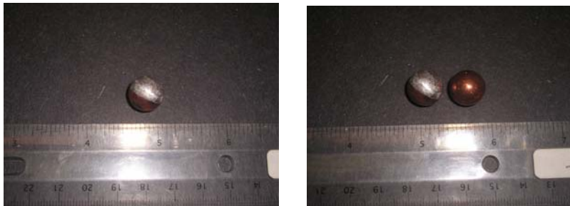
FIGURE 37. PROJECTILE WITH HEMISPHERICAL THIN FILM OF MELTED ALUMINUM FROM IMPACT (LEFT) COMPARED TO A NORMAL PROJECTILE (RIGHT)
