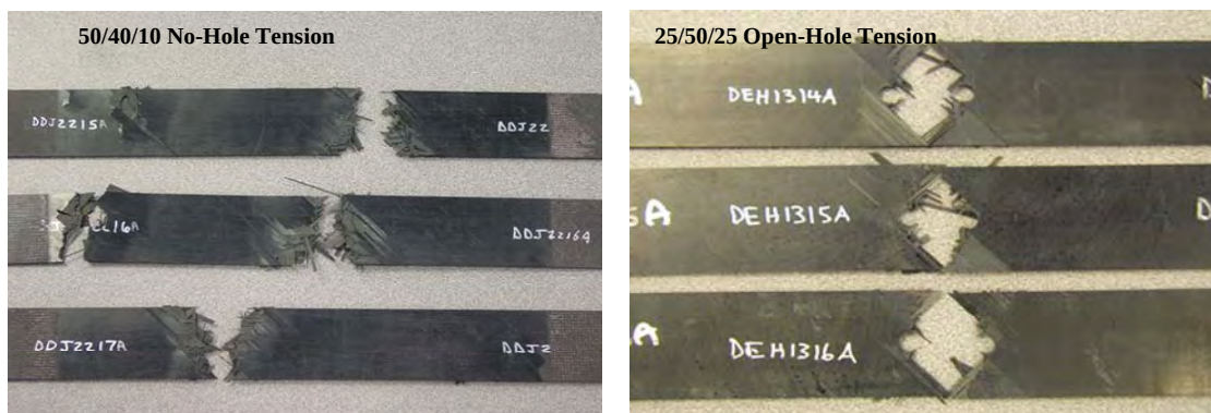
Figure 18. Typical Tension Failure Modes of Laminate Tension Tests
