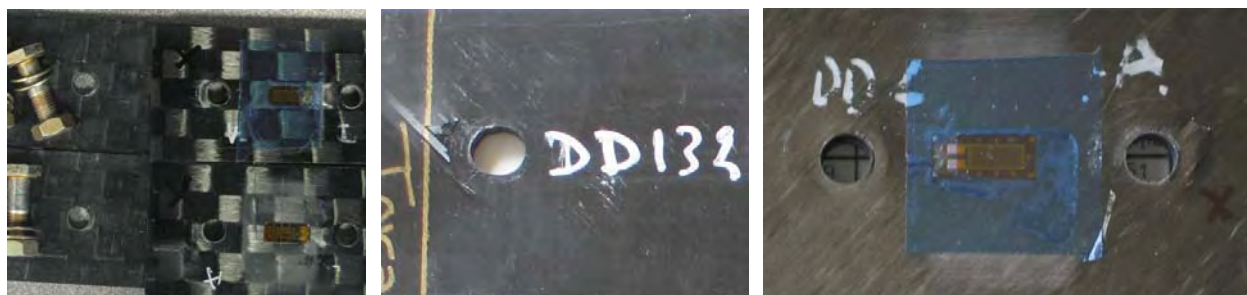
Figure 19. Localized Compression Failure of Laminate Bearing Tests
