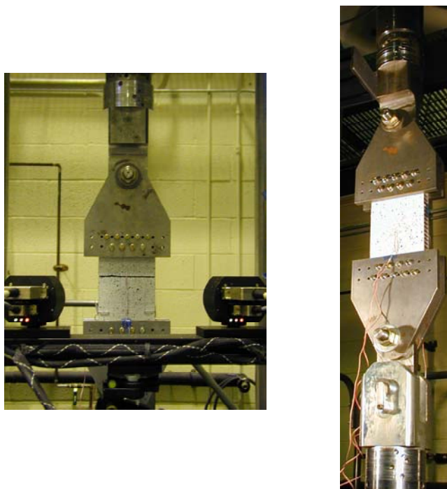
FIGURE 31. UNIDIRECTIONAL TENSION COUPON TEST SETUP
