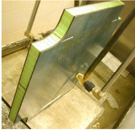
FIGURE 7. WICHITA STATE UNIVERSITY ULTRAPAC SCANNER (C-SCAN)
