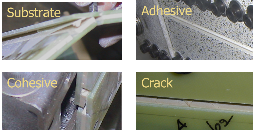
FIGURE 6-11. FAILURE MODES OF ES6292-FG7781 FLAT-JOINT SPECIMENS
