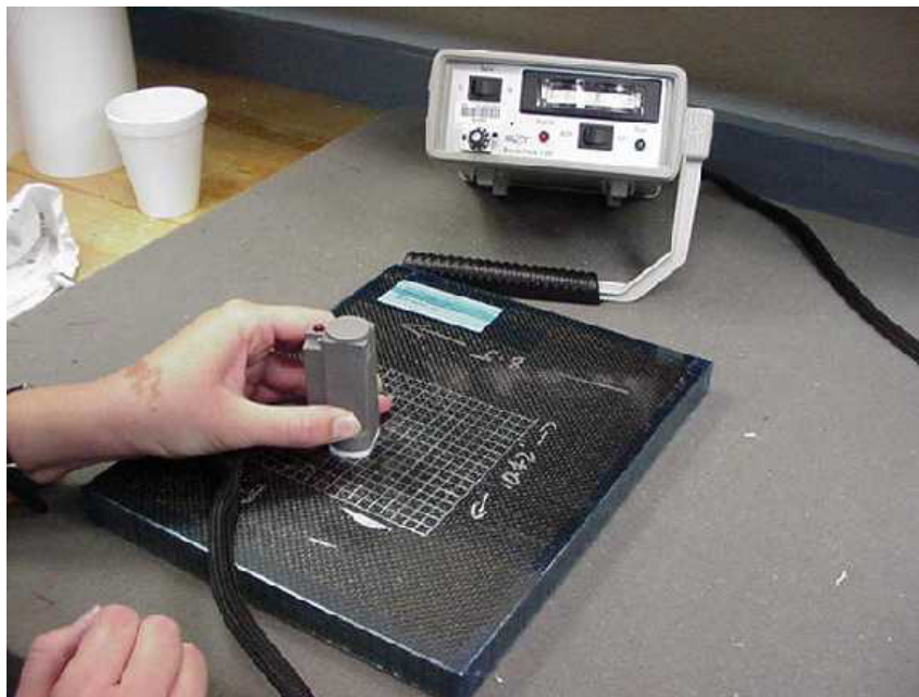
FIGURE 7. V-95 BOND TESTER USED FOR MECHANICAL IMPEDANCE ANALYSIS
