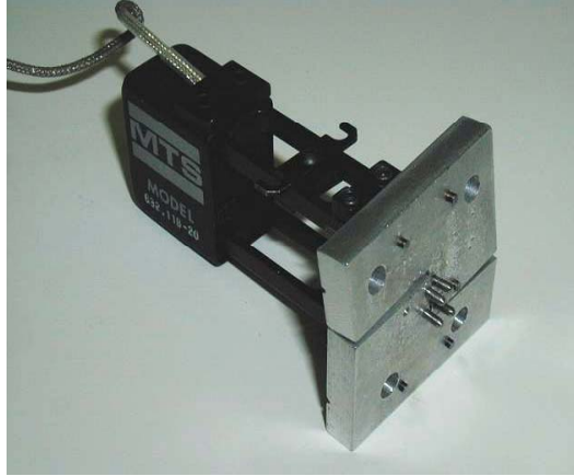
FIGURE 7. MODIFIED KGR-TYPE EXTENSOMETER (FOUR-PIN CONFIGURATION) FOR MEASURING ADHESIVE SHEAR STRAIN
