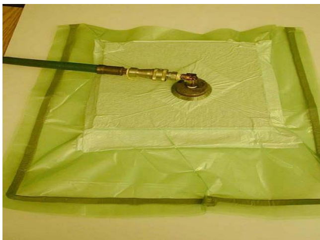
FIGURE 3. VACUUM BAGGING ADHESIVE TEST PANELS
