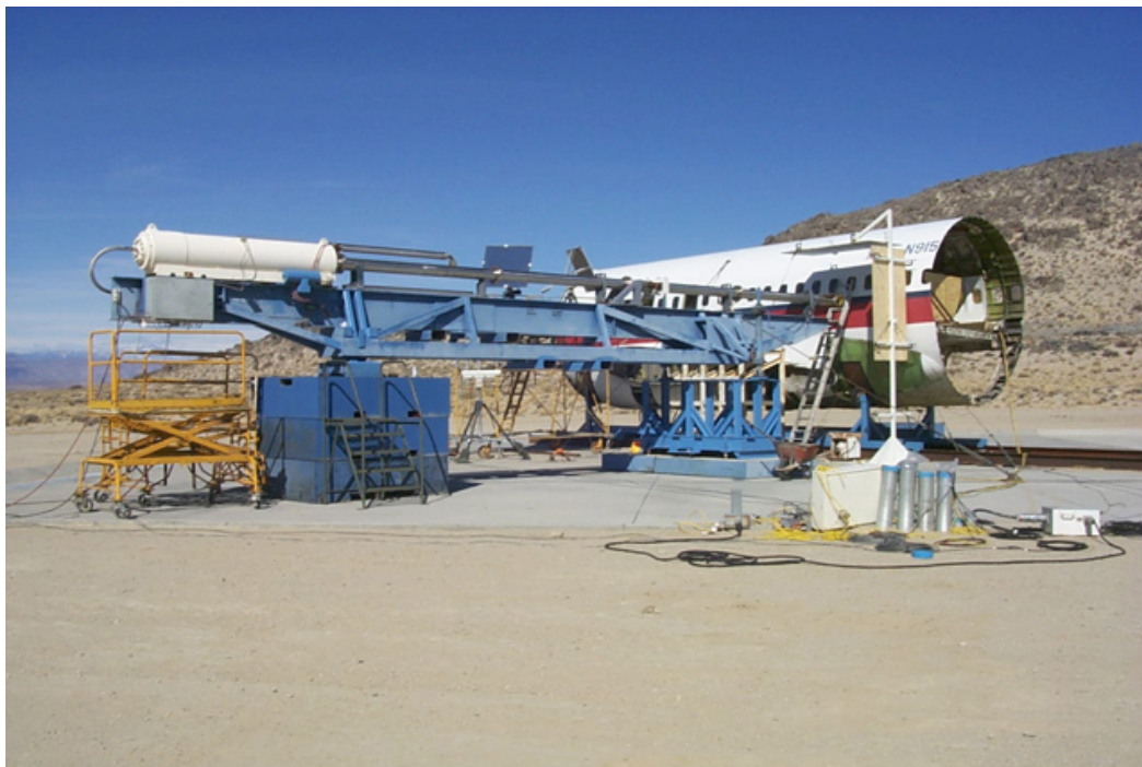
FIGURE 5. TEST SETUP SHOWING GAS GUN AND FUSELAGE
