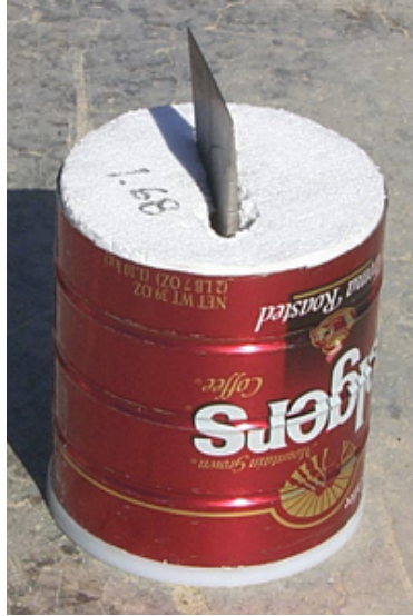
FIGURE 8. FINAL SABOT DESIGN WITH LOADED FRAGMENT
