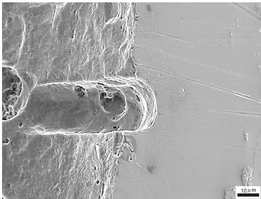
FIGURE 7-11. SEM MICROGRAPH OF A THROUGH SECTION OF A SHALLOW DAMAGE AT HOLE NO. 77 IN WING PANEL B3-2-5 OF THE CZ-184 AIRCRAFT SUGGESTING THAT THE CRACK WAS DISSOLVED BY CORROSION
