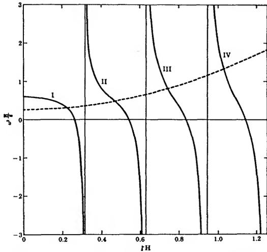
FIGURE 1.—Solution of dispersion relation for an isothermal atmosphere driven from below by an oscillating corrugation ( $\eta^2 < 0$ ). Abscissa:  $\zeta H$ , where  $\zeta$  is defined by equation (49). Ordinate: values of  $\omega^2 \frac{H}{g}$  derived from equations (39) and (49). The dotted line denotes the lower limit to values of the ordinate allowed by the condition  $\eta^2 < 0$ . Roman numerals denote consecutive branches of the solution.
