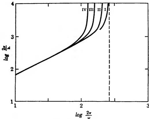
FIGURE 2.—Solution of dispersion relation ( $\eta^2 < 0$ ). Abscissa: wavelength of driving corrugation,  $2\pi/k$ . Ordinate: period of oscillation,  $2\pi/\omega$ . Dotted line shows the upper limit to the period.
