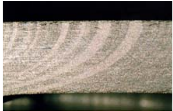
Fig. 47. Clearly defined fatigue crack arrest marks extending away from the initiation region.
