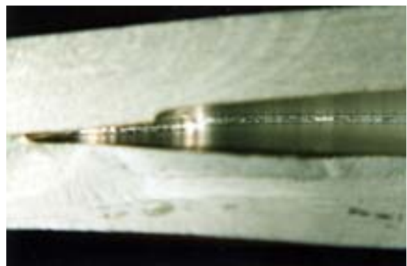
Fig. 44. Edges of the internal cavity, showing a continuous fillet of a metallic alloy.
