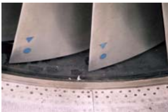
Fig. 30. Small fragment of blade debris found embedded within the fan attrition lining of the number-4 engine.
