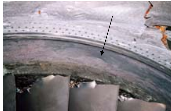
Fig. 6. Closer view of the blade primary impact point. Alignment with the blade pitch angle can be seen.
