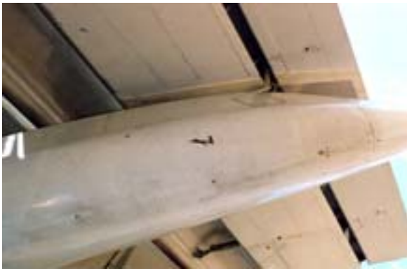
Fig. 33. Localised perforation and scoring of the number-five canoe fairing.
