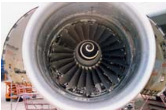
Fig. 1. General view into the intake of the number-3 engine of G-BNLD after the blade failure.
