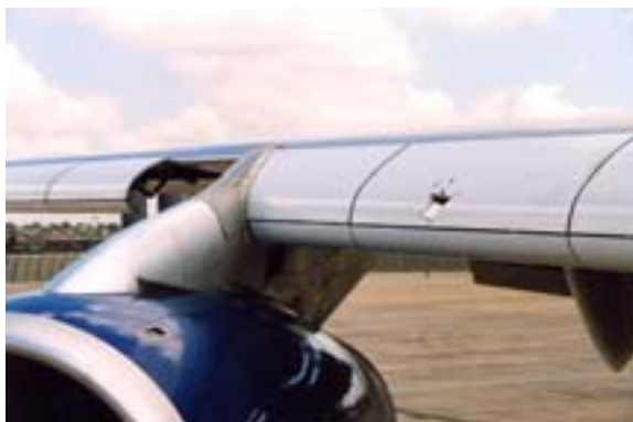
Fig. 31. Damage to the centre-section leading edge flap, right wing.
