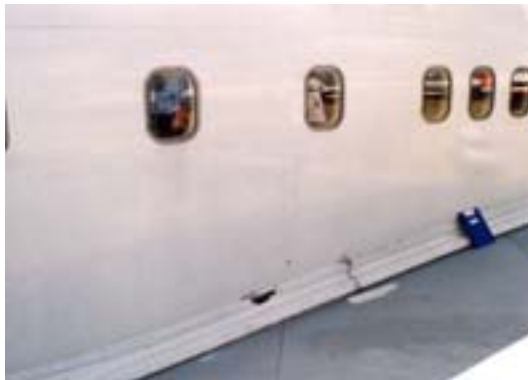
Figs. 34 (Left) & 35 (Right). Impact damage found on the fuselage and trim panels at station 1140, above the wing root.
