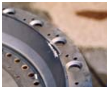
Fig. 7 Left - Fractured blade stub after removal of the annulus filler plates.
