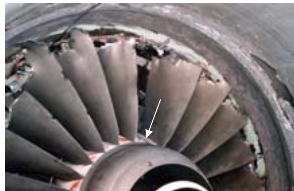
Fig. 2. Typical damage sustained by the engine fan (low-pressure compressor). Position of the failed blade is arrowed.
