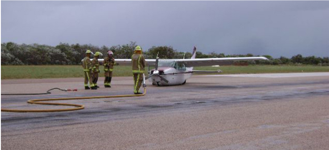
Collapsed landing gear involving a Cessna 210 Centurion (VH-PBV), at Broome Airport, Western Australia (ATSB investigation AO-2013-039)
