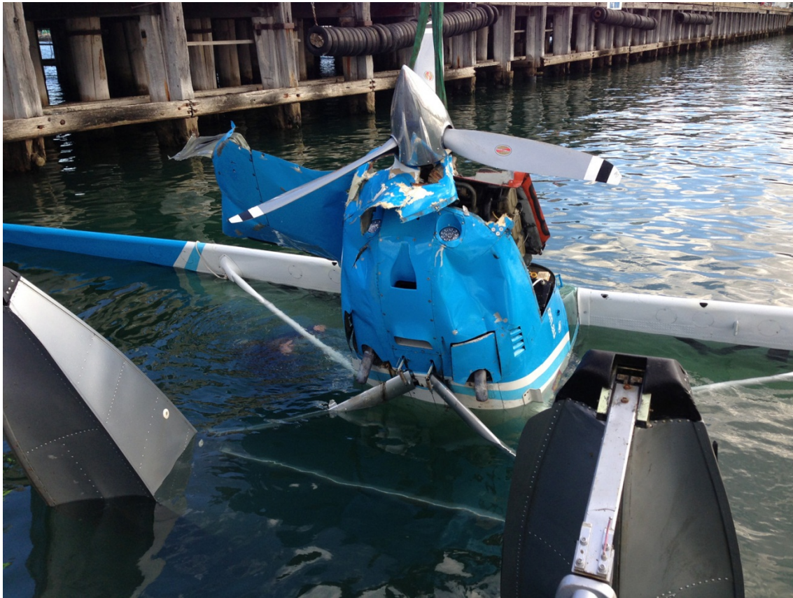
Wheels-down water landing involving a Cessna U206F Stationair floatplane (VH-UBI), Corio Bay, Victoria (ATSB investigation AO-2013-020)
