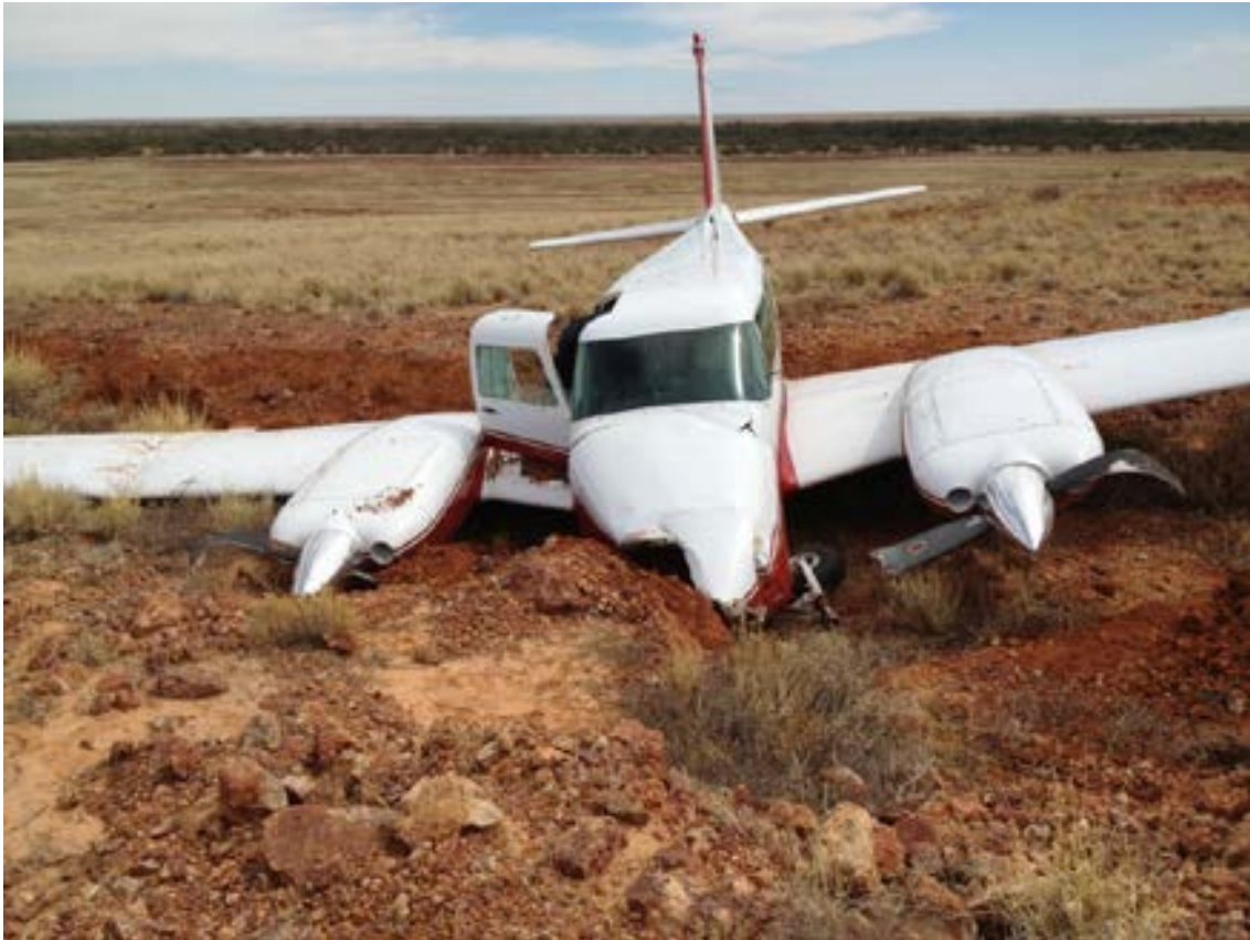
Runway excursion, Piper PA-39 Twin Comanche (VH-MMN), Innamincka Township authorised landing area, South Australia (ATSB investigation AO-2012-146)
