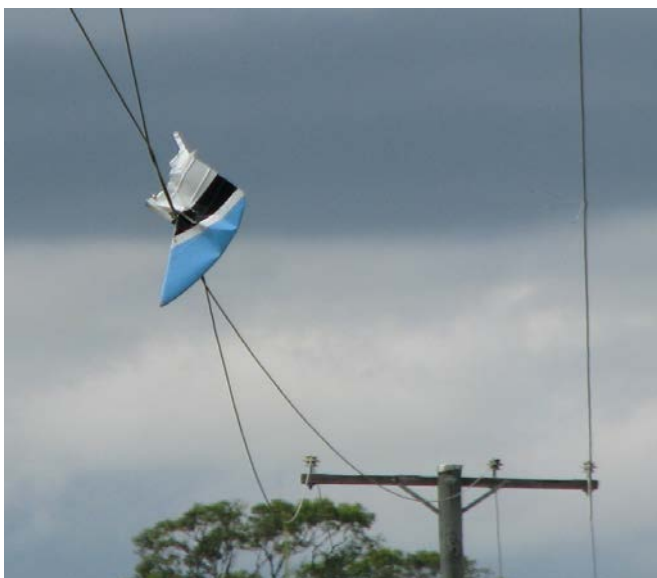
Electricity conductors and detached rudder horn (Investigation AO-2010-026)
