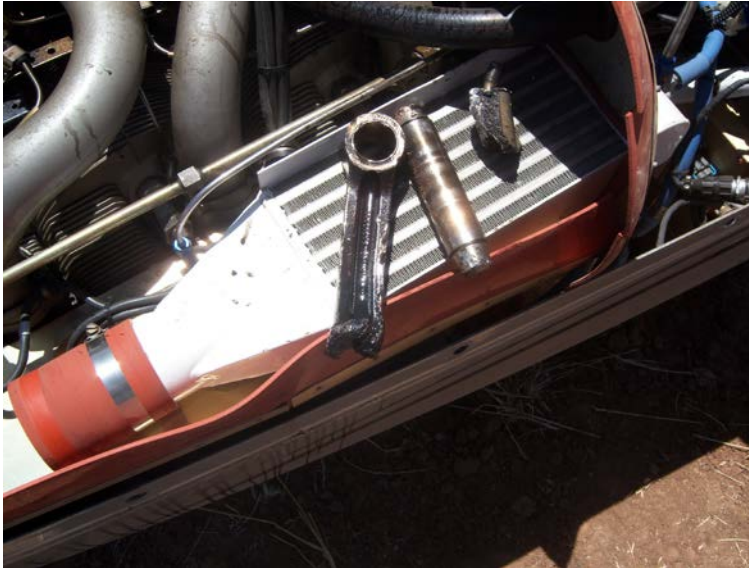
Figure 3: Engine number two cylinder failed parts
