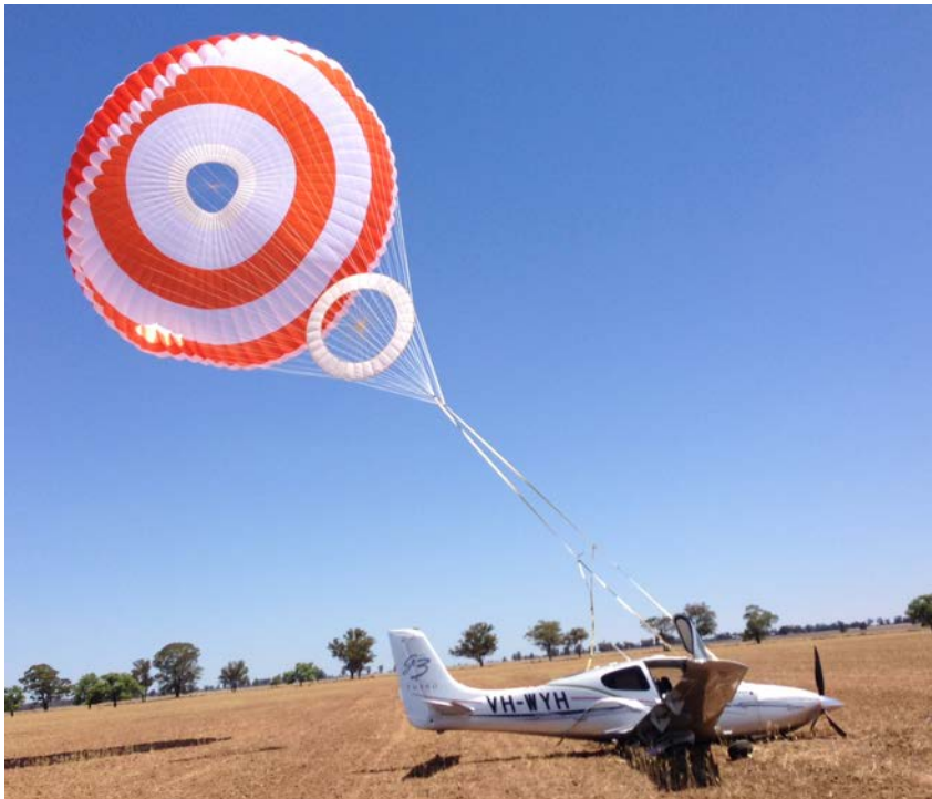
Figure 1: Parachute inflated at accident site
