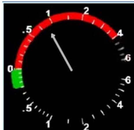
Figure 4: Illustration only of VSI with TCAS lights
