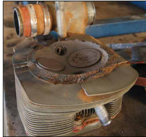
Figure 3: Failed number-4 cylinder
