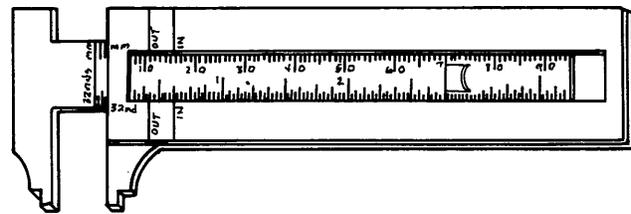
**Figure 3-28. Slide Caliper**
