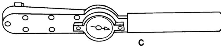
Figure 8-9. Type II, Style A Torque Wrench - Rigid Case with Indicator Dial (Direct Reading)
