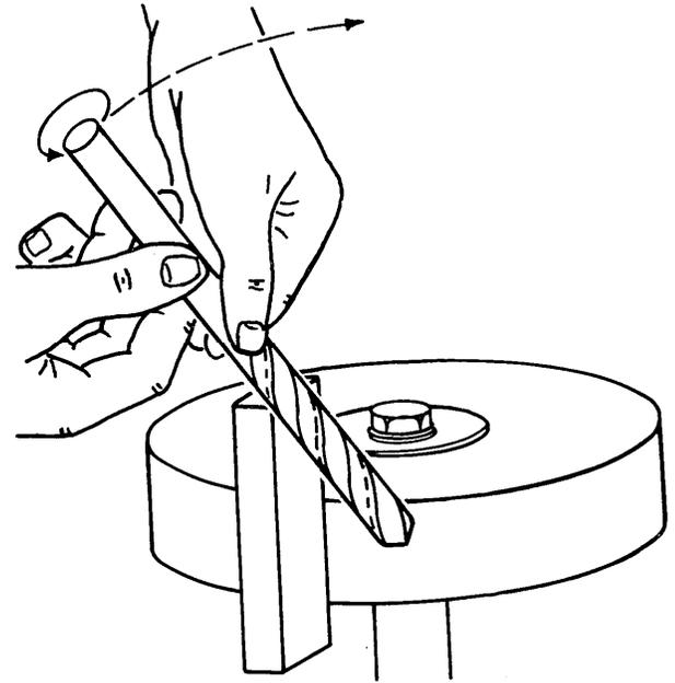
**Figure 4-88. Hand Grinding of Heel to Cutting Edge**
