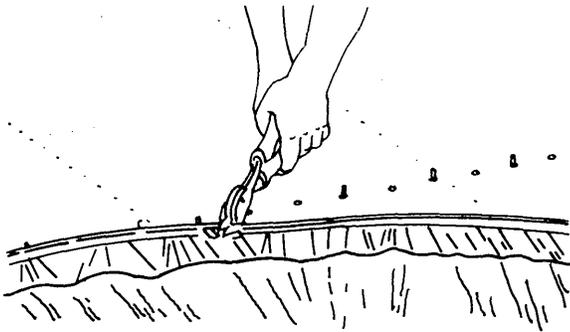
Figure 7-17. Using Deicer Boot Pliers
