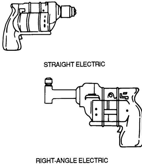
**Figure 6-2. Electric Drills**
