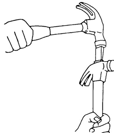
**Figure 4-12. Installing Wedge**
