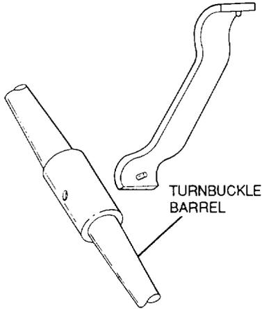
Figure 7-8. Turnbuckle Wrench
