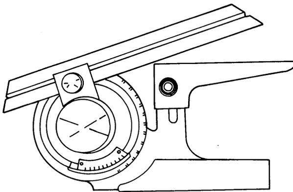
**Figure 3-12. Bevel Protractor**
