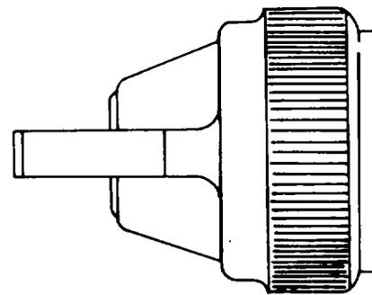
Figure 5-3. Nozzle Position to Produce Vertical Fan
