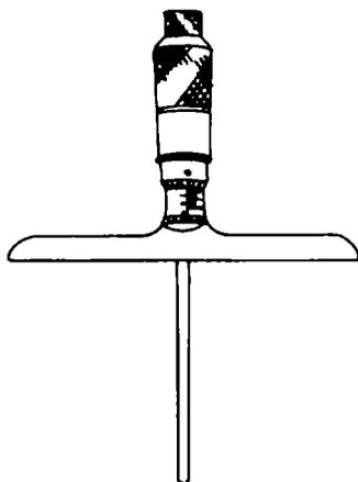
Figure 3-36. Depth Micrometer
