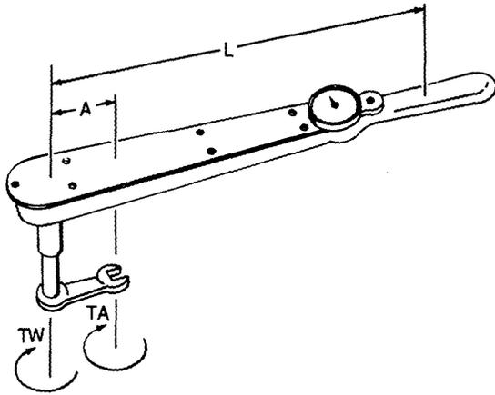
TW = INDICATED TORQUE VALUE ON TORQUE WRENCH
