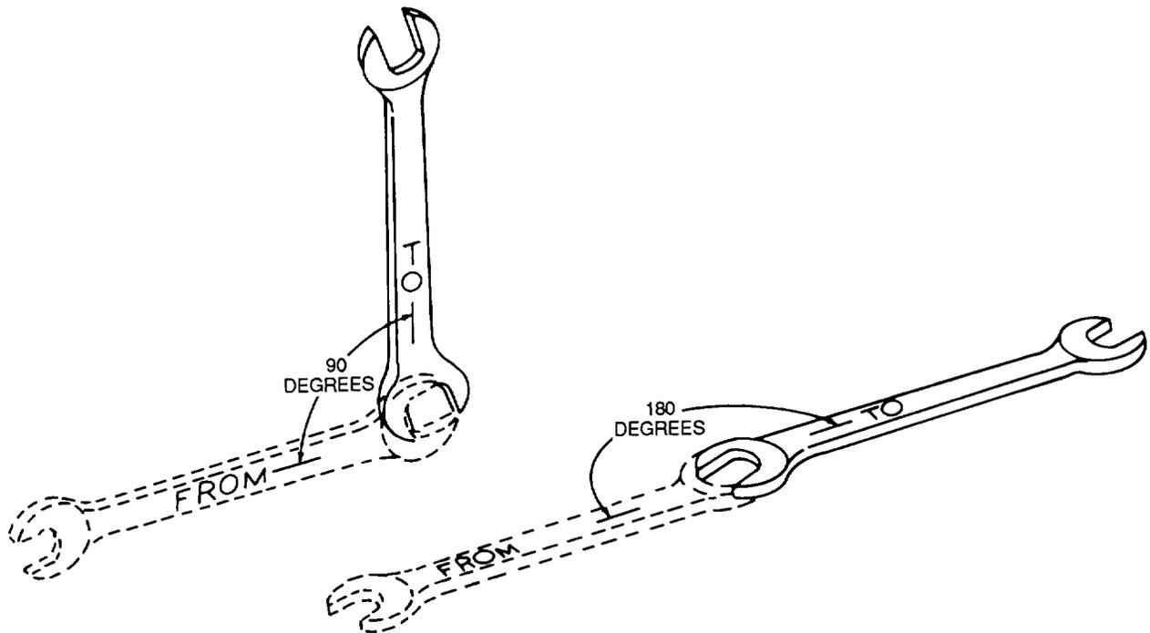
Figure 8-28. Tightening to 90- or 180-Degree Wrench Arc
