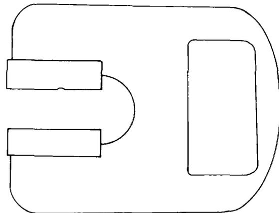
Figure 3-59. Snap Gauges
