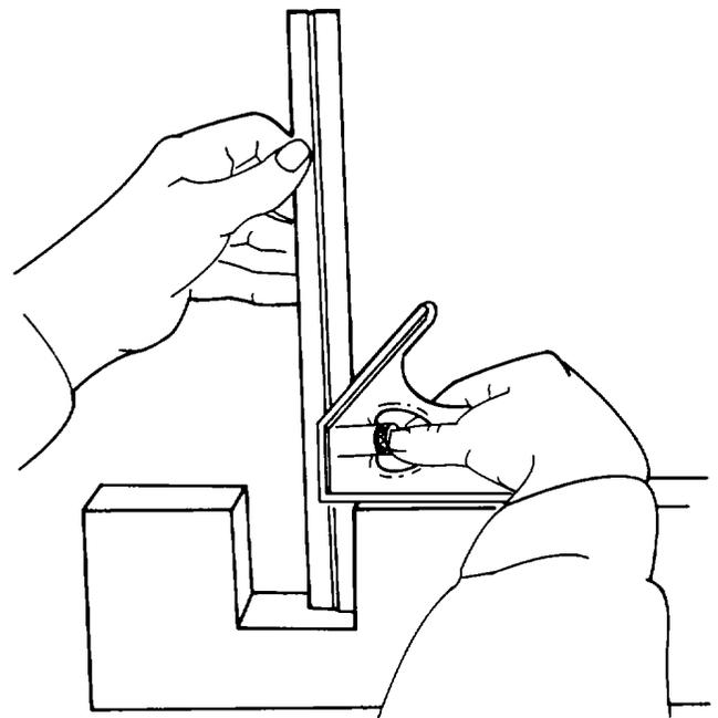
Figure 3-20. Determining Depth with the Square Head
