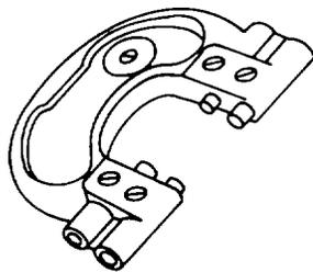
**Figure 3-62. Snap Gauge for Checking Dimension Between Surfaces**
