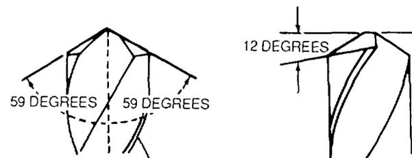
**Figure 4-86. Usual Cutting Edge and Heel Angles**
