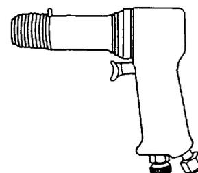
Figure 5-17. Pneumatic Hammer
