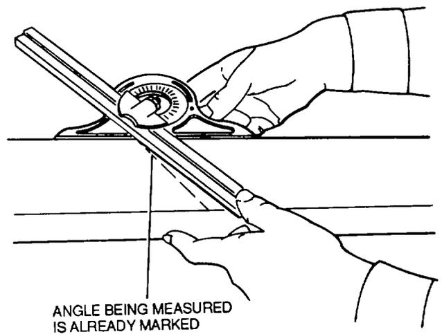
Figure 3-19. Checking Angle
