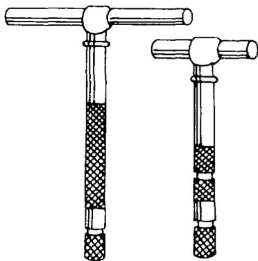
Figure 3-77. Telescoping Gauges
