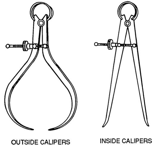
Figure 3-25. Spring-Joint Calipers
