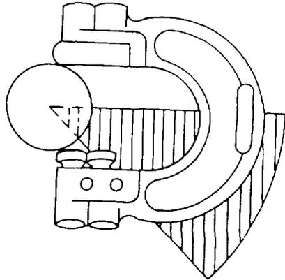
Figure 3-67. Placing Snap Gauge on Cylindrical Part
