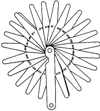
Figure 3-70. Thickness Gauge
