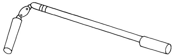
Figure 7-14. Telescoping Magnet
