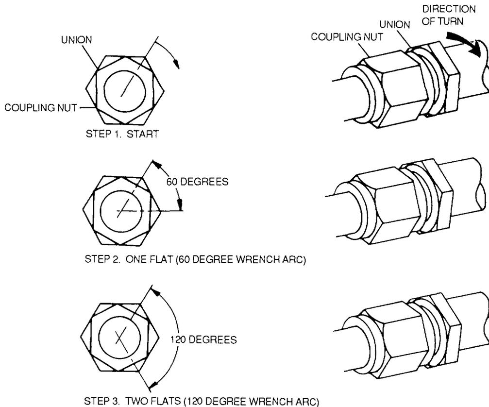
**Figure 8-26. Tightening to 60- or 120-Degree Wrench Arc**
