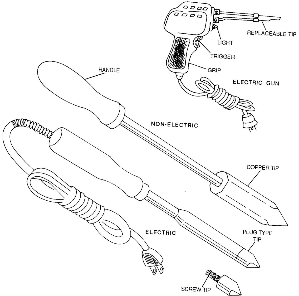
Figure 7-22. Soldering Tools
