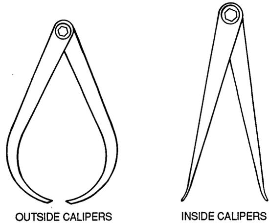
Figure 3-24. Simple Calipers
