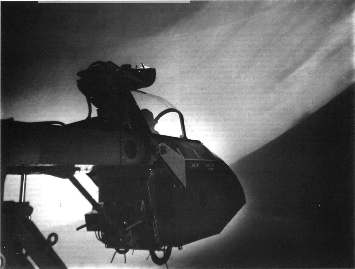
FIG. 1. Visual display produced by skyscape projector to represent flight at altitude.
