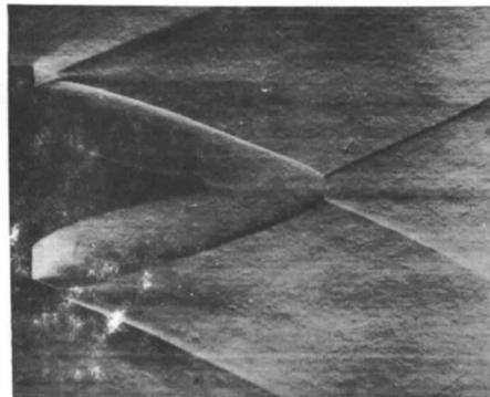
FIG. 25. Schlieren photographs showing the effect of jet pressure ratio on the flow field.
