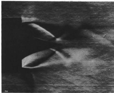
FIG. 20. Schlieren photographs showing the effect of jet pressure ratio on the flow field.
