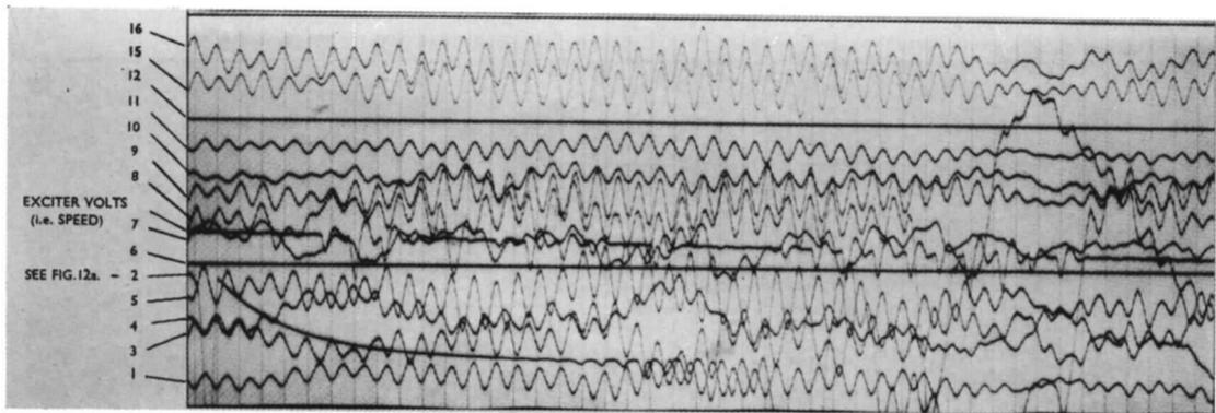
FIG. 12b. 10.7 c.p.s. resonance at 350 knots, 10 lb in. exciter moment.
