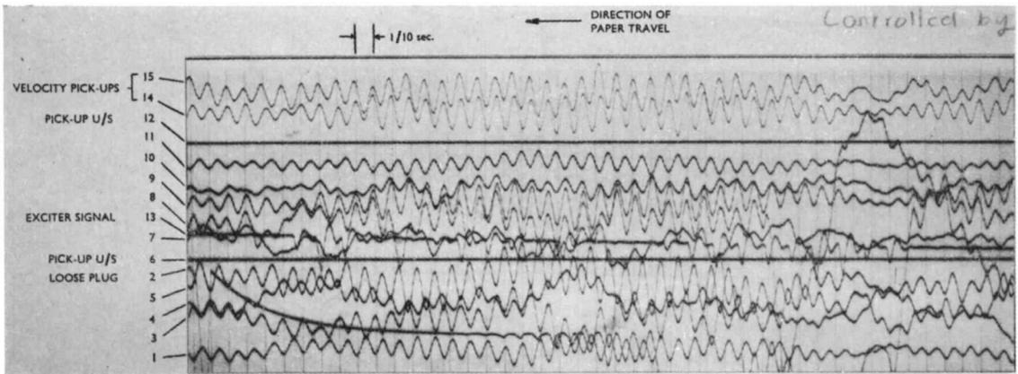
FIG. 2a. Sweep through 10.5 c.p.s. resonance at 350 knots.
