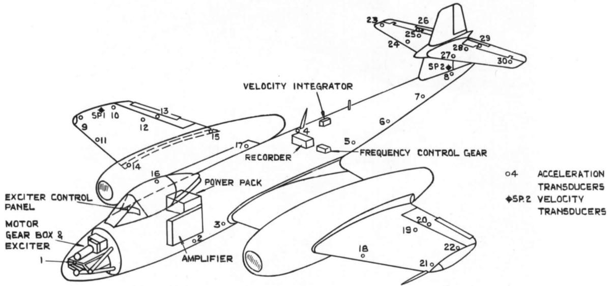
FIG. 1. Layout of experimental equipment in WK 878.
