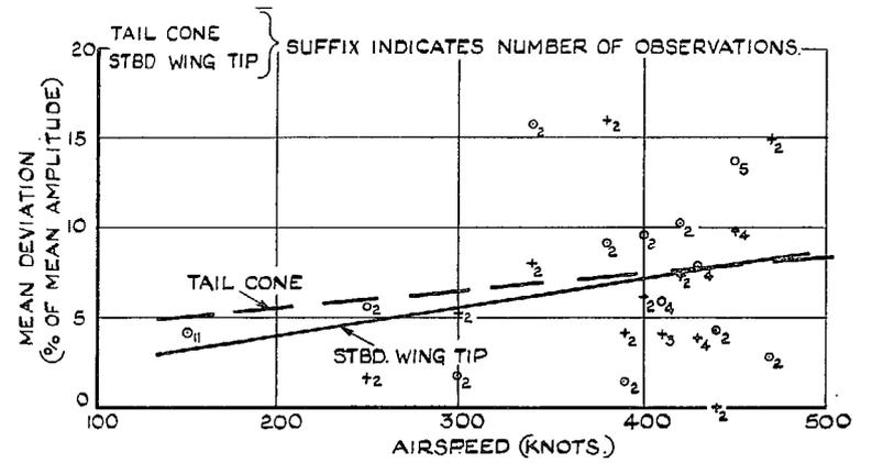
FIG. 6. Effect of airspeed on the scatter of resonant amplitudes measured in the 10.5 c.p.s. mode.
