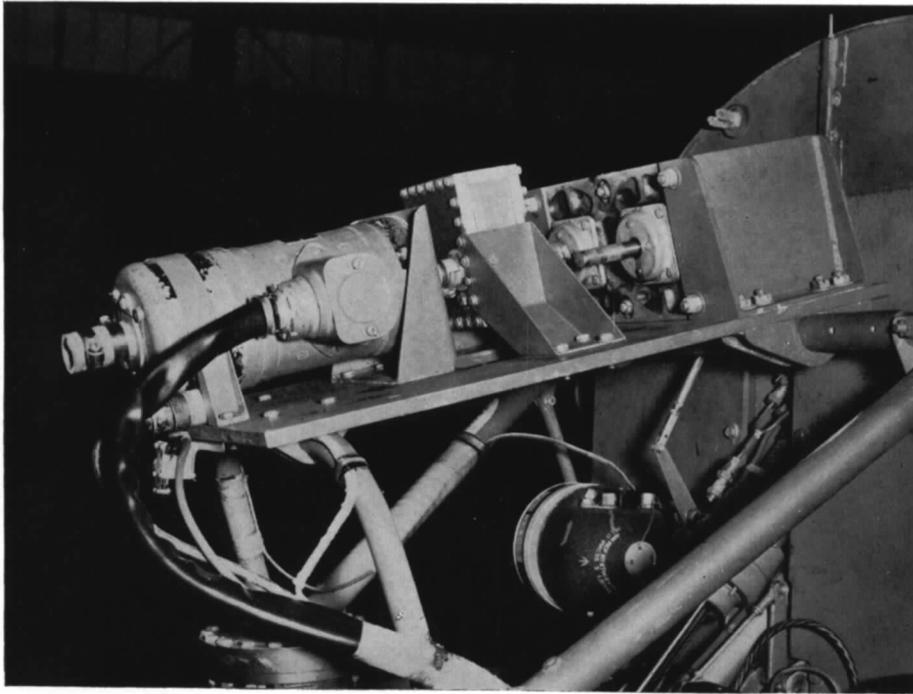
FIG. 4. Installation of motor, gear-box and exciter.
