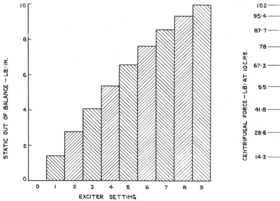
FIG. 5. Characteristics of R.A.E. 10 lb in. linear inertia exciter.
