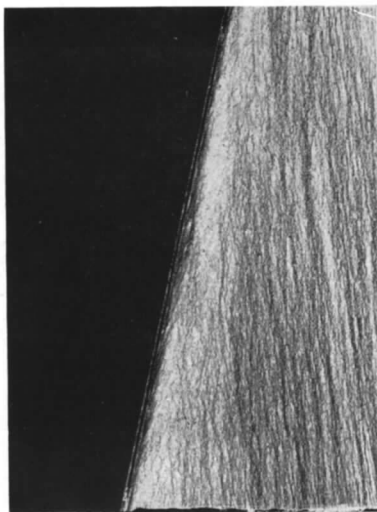
FIG. 5. Wing B. Oil-flow patterns at low incidences.
