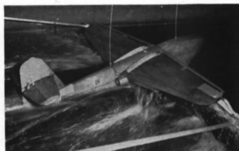
FIG. 24. Take-off at overload 17,250 lb. Seaworthiness tests.
