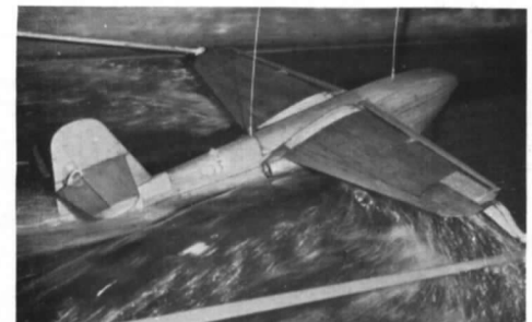
FIG. 23. Take-off at normal load 15,200 lb. Seaworthiness tests.
