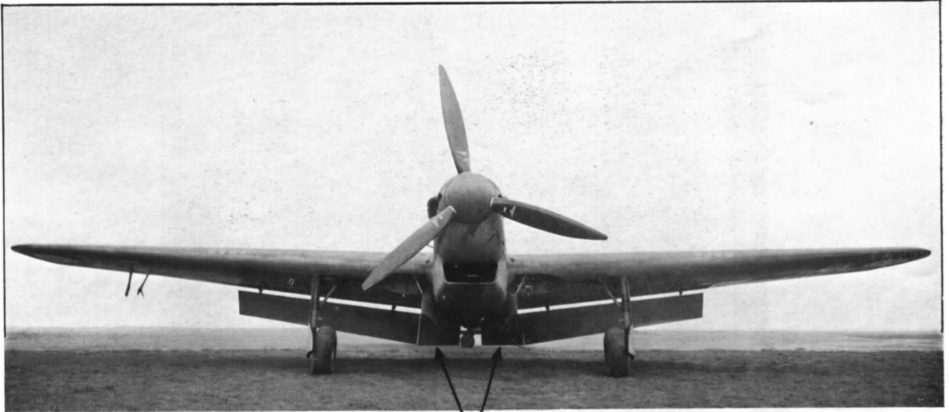
ADDED FLAP AREA AT CENTRE SECTION
