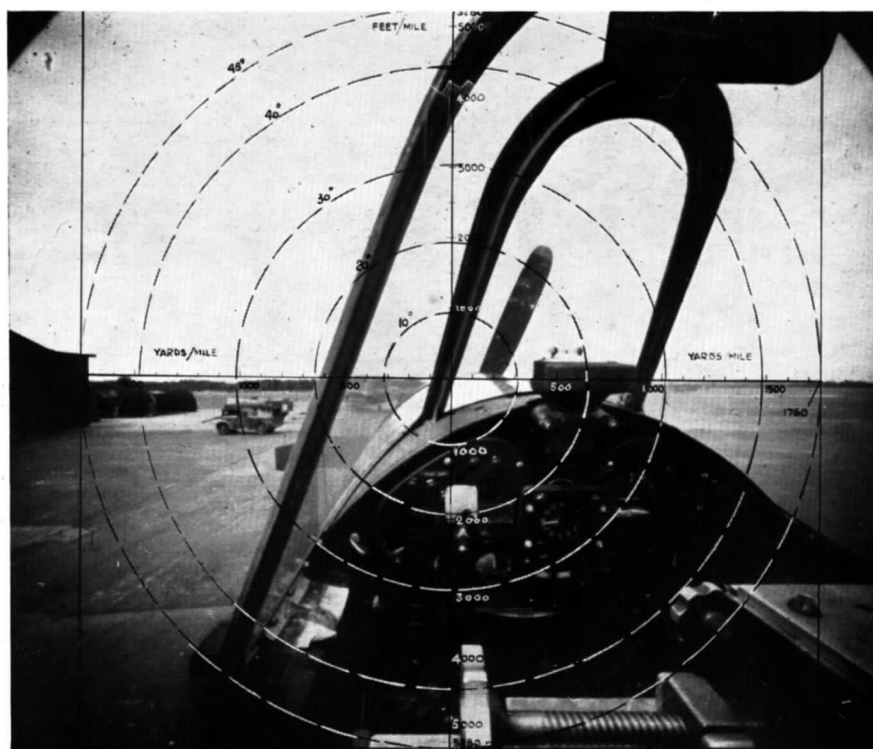
Photograph B. Camera position corresponding to pilot's left eye when seated with head moved 4.7 inches from central position, seat fully up. Centre of graticule corresponds to a direction of sight inclined down at 10.3^\circ to wing chord.
