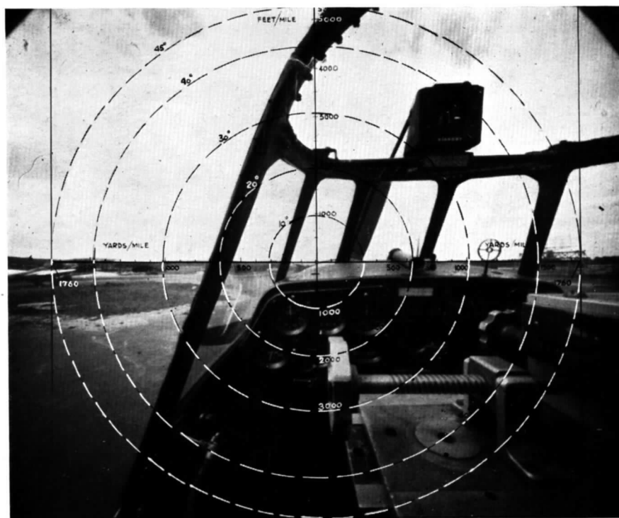
Photograph B. Camera position corresponding to pilot's left eye when seated with head moved 5\frac{1}{4} inches from central position, seat fully up. Centre of graticule corresponds to a direction of sight inclined down at 13.3^\circ to wing chord.
