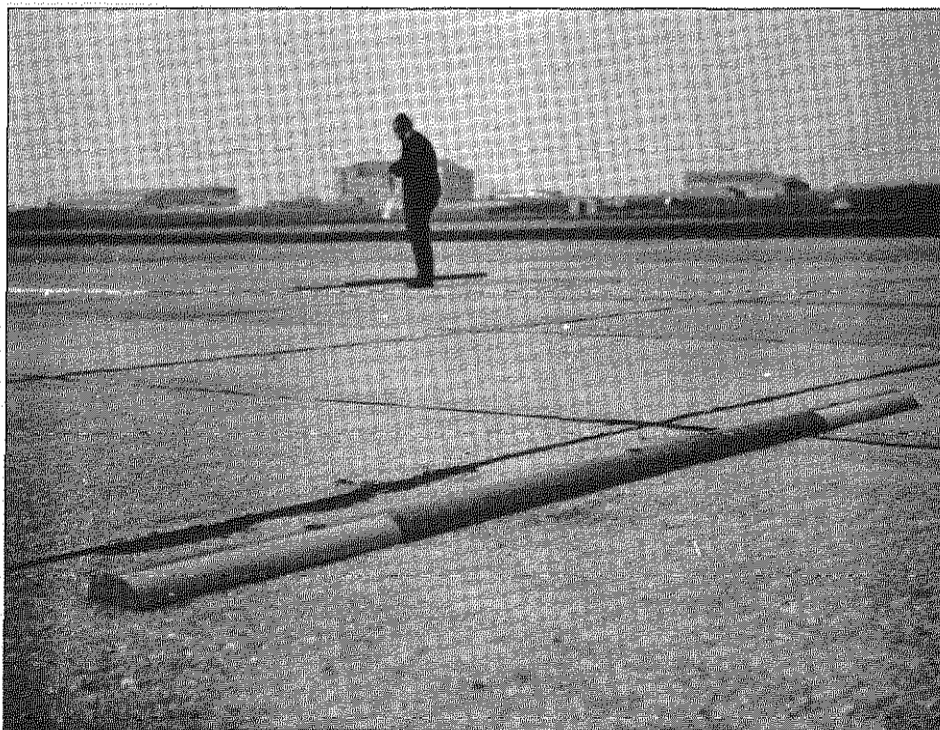
FIG. 31. SIMULATED 3 INCH BUMPS.
