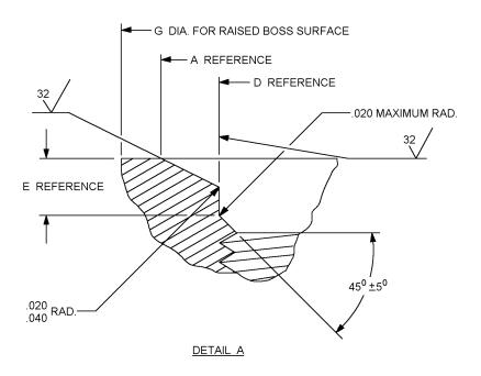
FIGURE 1. Bosses, standard dimensions for gasket seal straight thread.
