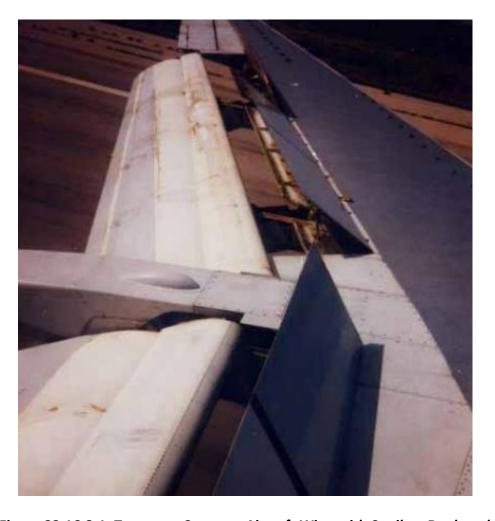
Figure 22.16.8-1: Transport Category Aircraft Wing with Spoilers Deployed (FAA-H-8083-31, 2012)
