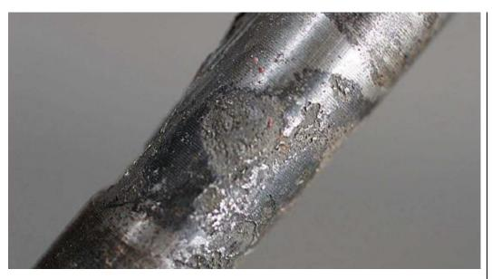
Figure 4.4.2-3: Dissimilar Metal (Galvanic) Corrosion\_(FAA-H-8083-30, 2008)
