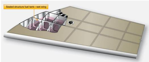
Figure 22.16.2-17: Fuel Region in Wing Structure (FAA-H-8083-31, 2012)
