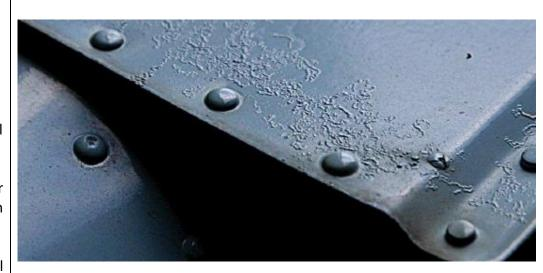
Figure 4.4.2-2: Filiform Surface Corrosion\_(FAA-H-8083-30, 2008)
