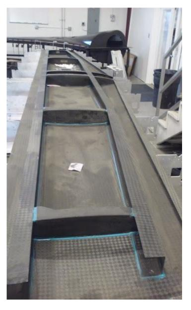
Figure 22.12.2-4: Internal Structure of a General Aviation wComposite
