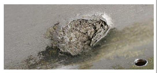
Figure 4.4.2-4: Intergranular Corrosion Shown as Exfoliation\_(FAA-H-8083-30, 2008)
