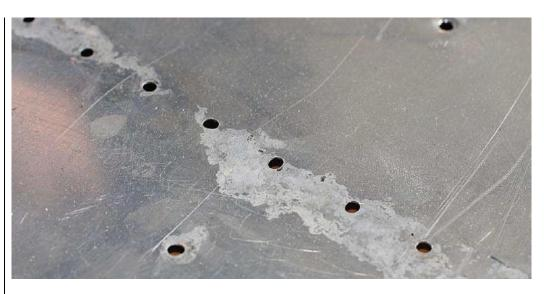
Figure 4.4.2-1: Surface Corrosion\_(FAA-H-8083-30, 2008)
