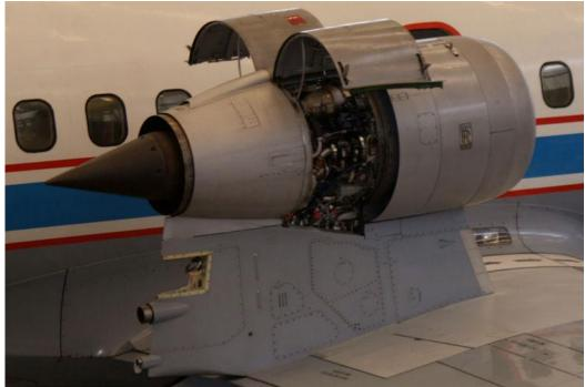
Figure 22.12.2-5: Cowling on Transport Category Turbine Engine Nacelle (Courtesy Wikimedia Commons)
