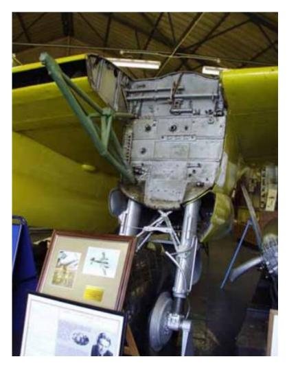
Figure 22.12.2-1: An Engine Nacelle Firewall\_(FAA-H-8083-31, 2012)
