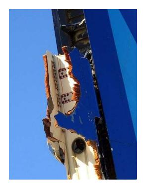
Figure 4.1.3-8: Sandwich Composite Rudder Failure due to Water Ingress (Source: <u>Aero News Network</u>)
