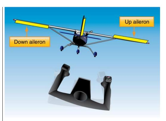
Figure 22.16.7-2: Yoke and Relative Aileron Movements (FAA-H-8083-31, 2012)
