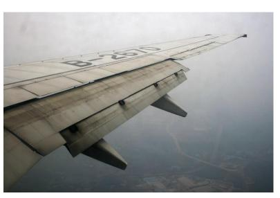
Figure 22.16.4-1: Various Flaps on Different Aircraft (Courtesy Wikimedia Commons)
