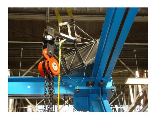
Figure 22.12.2-2: A 4130 Welded Steel Engine Mount for a Part 23 Aircraft Undergoing Certification Structural Testing (Author's Collection)
