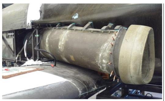
Figure 22.12.2-6 Air Intake Duct and Lip for Fuselage Internal Mounted Engine (Author's Collection - Courtesy of Stratos Aircraft)
