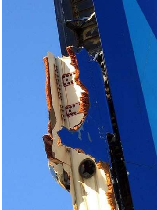
Figure 4.1.3-7: Sandwich Composite Rudder Failure due to Water Ingress (Source: Aero News Network )
