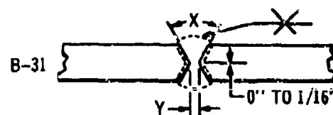
(C) DOUBLE-V BUTT JOINT, WELDED BOTH SIDES
