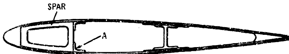
Figure 17-11. Typical Rotor Blade Design — Alternate 2
