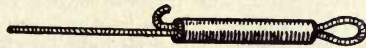
Fig. 106.—The Voisin method of making eyes by passing the end of the wire twice through a piece of copper tube, leaving an eye, and bending the end of the wire over.
