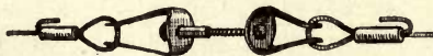
Fig. 140.—A simple rigging screw made out of a short cycle spoke and nipple, and two strips of metal.
