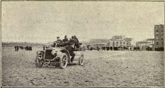
Fig. 54.—Experiments at Issy with a glider in 1900, power being obtained by towing the glider with a car.
