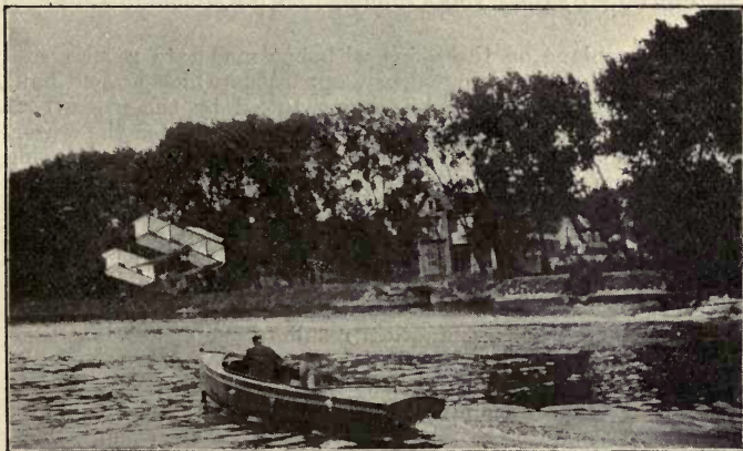
Fig. 57.—Gabriel Voisin in his glider towed over the Seine by a fast motor-boat.
