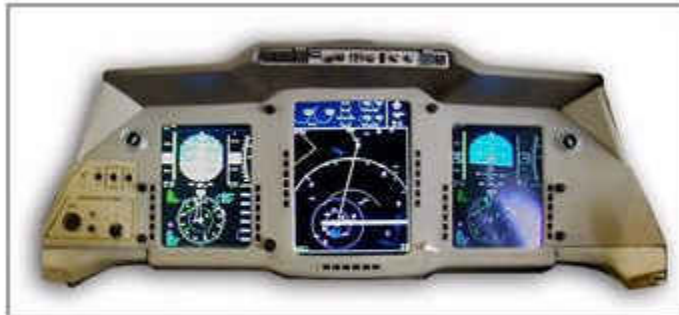
The cockpit in the Eclipse 500 interior mock-up has the standard equipment PFD (left), MFD (center), and optional PFD (right).
