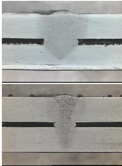
Figure 3: Gap bridging capability of the laser plus MIG welding process. Between 8 kW and 10 kW of CO 2 laser power was used and feed rates reached 5 m/min. Source: Fraunhofer Center for Laser Technology.
