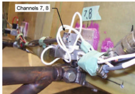
Fig. 9 – Lower Left Accelerometer Installations
