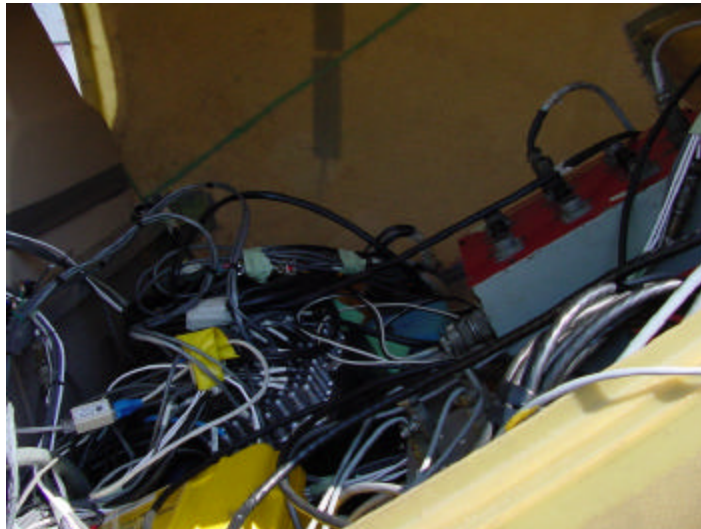
Fig. 27 – Onboard Instrumentation (Aircraft baggage compartment containing data acquisition and pyrotechnics equipment)
