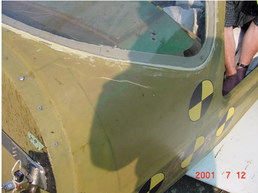
Fig. 38 – Photo – Fuselage (Wrinkle under Windshield)
