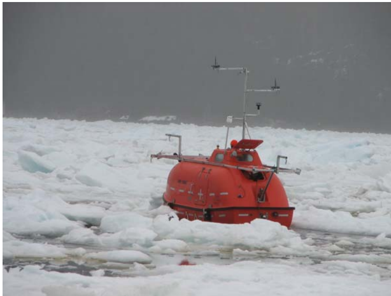
Figure 1-1: TEMPSC Testing in Ice.
