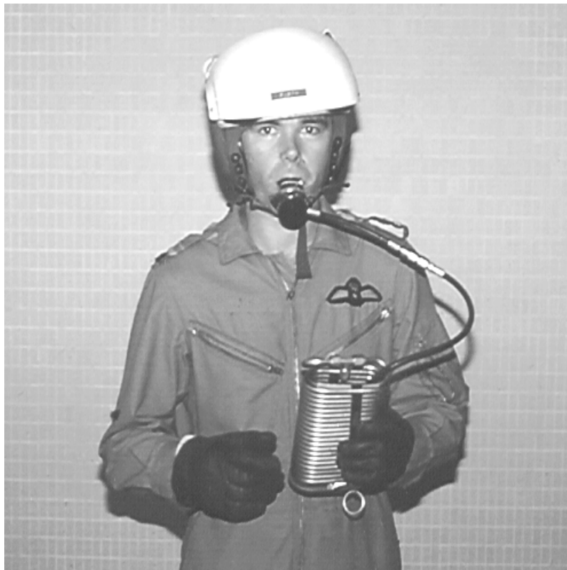
Figure 6b – The Robertshaw Controls Co. Unit. Unit is being demonstrated to show the bulk of the unit and impracticality of mounting on the lifejacket.
