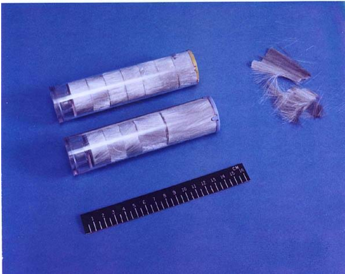
Figure 3-18: Typical Chaff Rounds and Chaff Dipoles – (U.S. Navy Photo).
