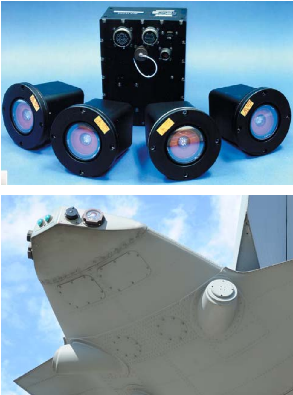
Figure 2-16: Top: AN/AAR-54 Electronic Unit and Sensors – (Courtesy of Northrop Grumman Corp.); Bottom: Aft Missile Warning Sensor Installation on a C-130 – (USAF Photo).
