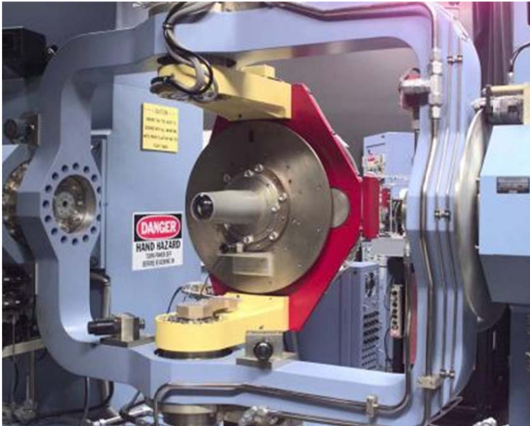
Figure 3-16: IR-Guided Missile Seeker Mounted on Full Motion Simulator – (U.S. DoD Photo).
