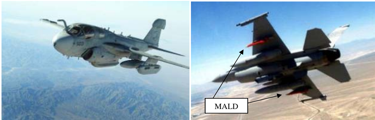
Figure 3-8: a) EA-6B Aircraft with External Jamming Pods; b) Miniature Air Launched Decoy Carried by F-16 – (U.S. DoD Photos).
