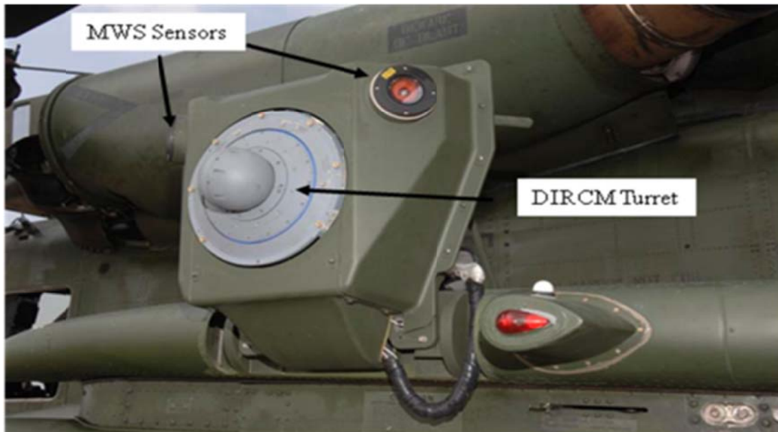
Figure 3-14: Department of the Navy Large Aircraft Infrared Countermeasures Installation on a CH-53E Helicopter – (U.S. Naval Air System Command Photo).
