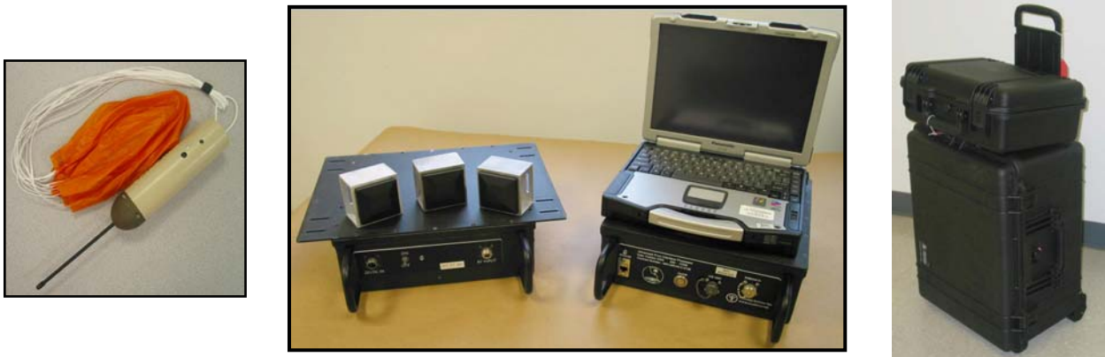
Figure 1: JPADS-MP Fly-Away Kit. (From Right to Left: Dropsonde, JPADS-MP Hardware, Laptop, and Carrying Case)
