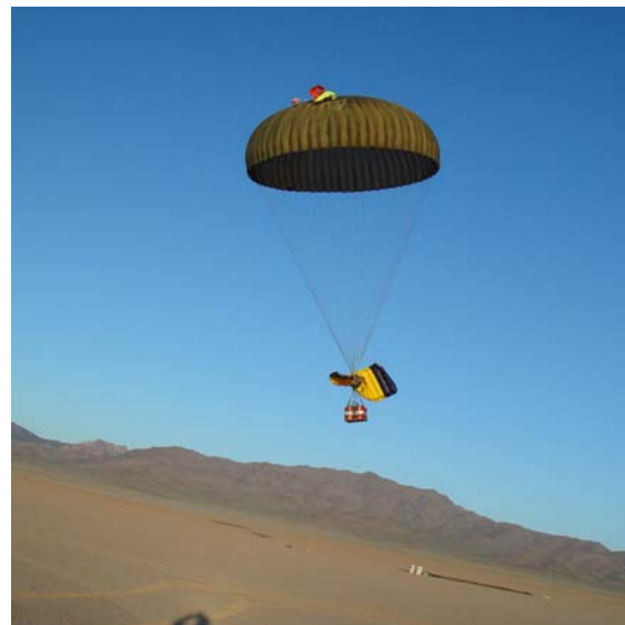
Figure 6: 2,000-pound CDS Payload SCREAMER System Transition from Guided Flight to Recovery Chute Landing.
