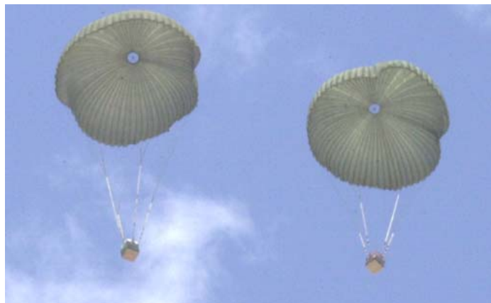
Figure 9: Two AGAS Systems in Flight and During a Double and Single Riser Slip.
