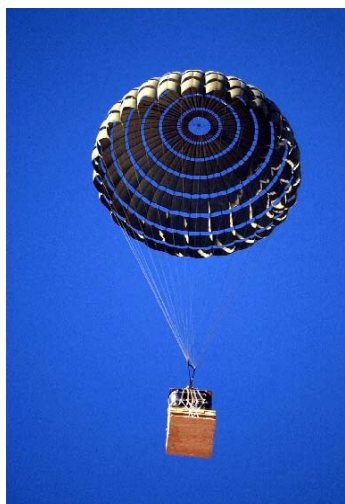
Figure 2: JPADS-MP Deployed 26-Foot Ring Slot CDS Drop.
