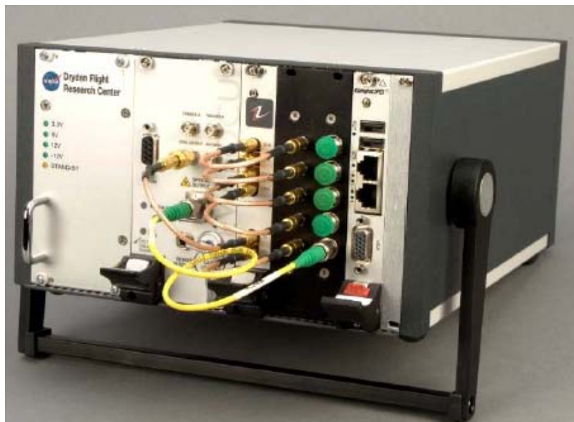
Figure 3-1: Ground-Based 4-Fiber Interrogation System.
